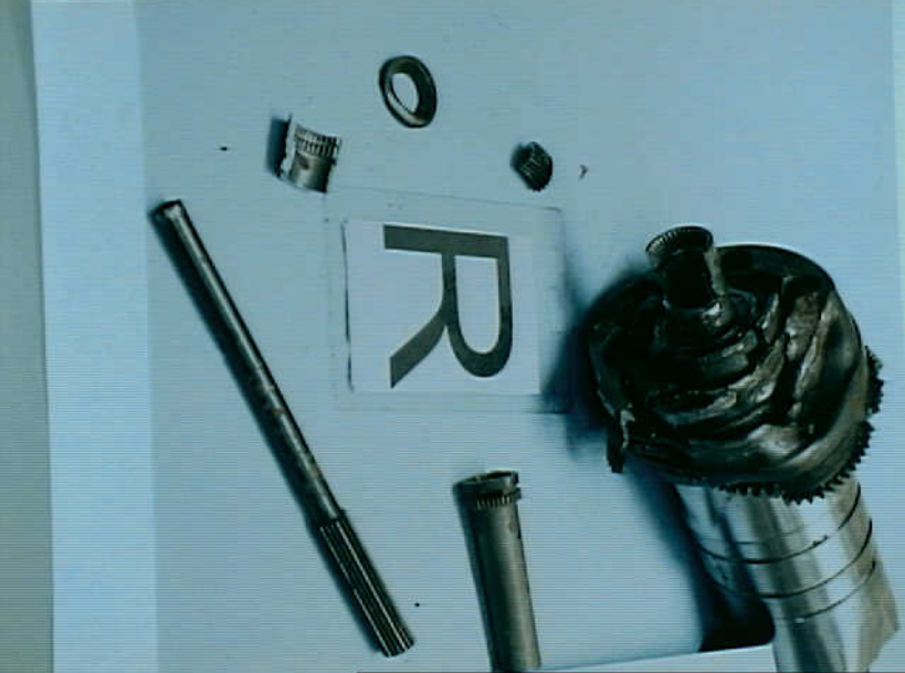
Powerplants 8 - Photo 26. Right propeller servo piston sectioned ball screw showing internal splines, and the external splines on the quill and transfer tube
