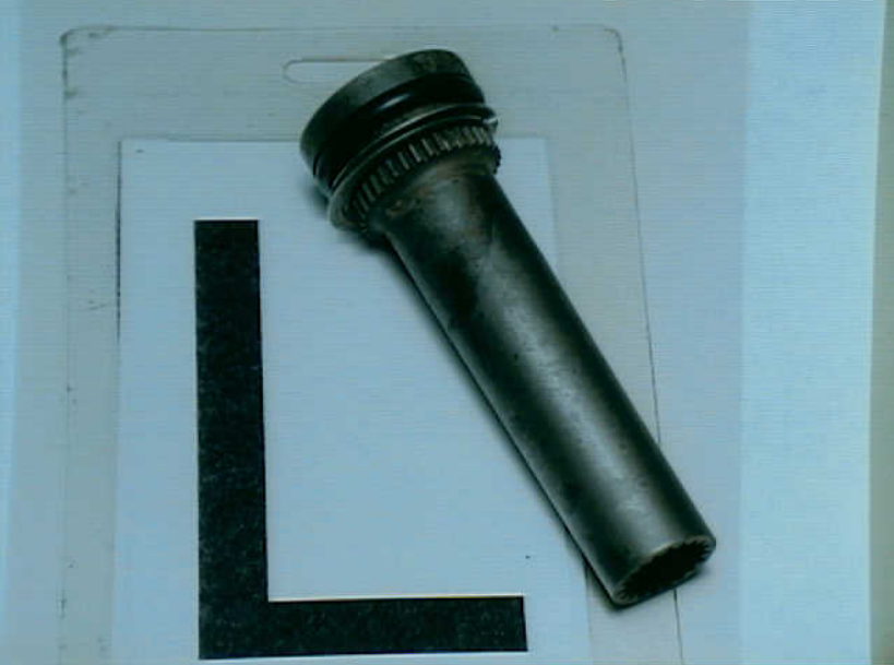
Powerplants 8 - Photo 25. Left propeller servo piston quill external and internal splines
