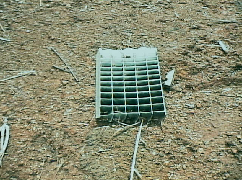
Powerplants 8 - Photo 23. Thrust reverser cascade found near No. 1 engine
