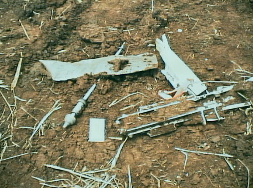
Powerplants 8 - Photo 22. Thrust reverser actuator jackscrew found near No. 1 engine
