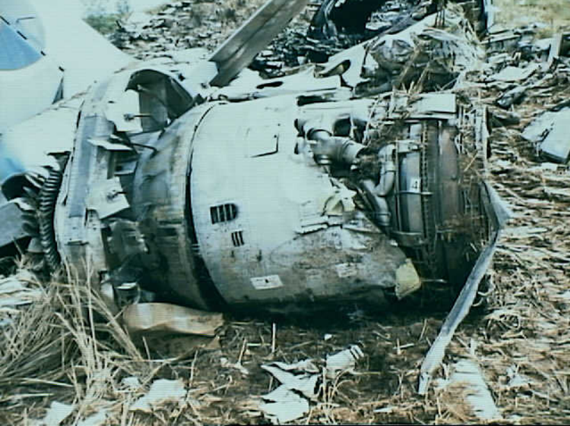
Powerplants 8 - Photo 20. No. 4 engine bottom and LPC
