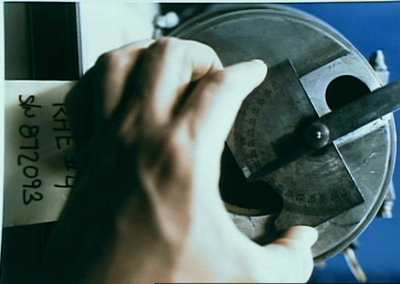
Powerplants 8 - Photo 20. Butt end of right hand propeller blade No. 4 showing measurement of witness mark on blade pin plateau with protractor to determine propeller blade pitch angle
