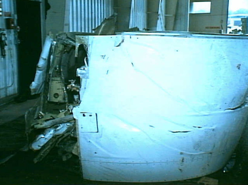
Powerplants 8 - Photo 2. Engine No. 1 inlet cowling, upper left side.
