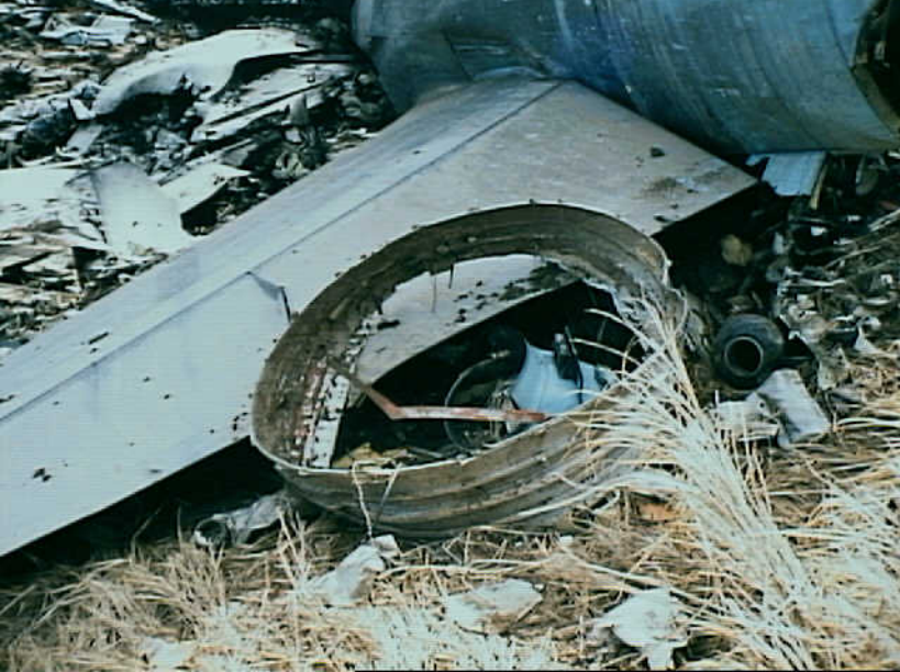
Powerplants 8 - Photo 18. No. 4 engine fan ring
