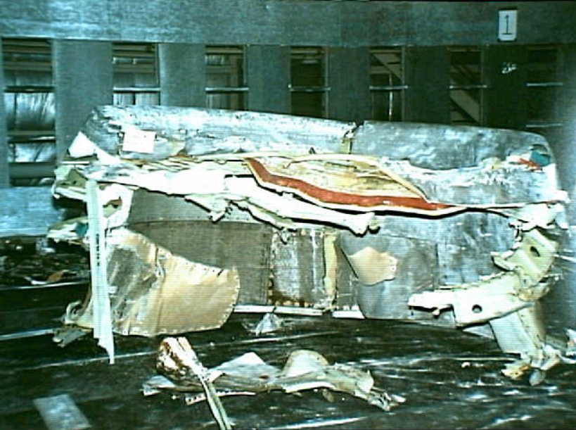
Powerplants 8 - Photo 18. Engine No. 2, inlet duct, left side.
