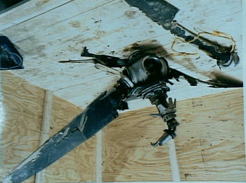
Powerplants 8 - Photo 16. Right propeller assembly as received at Hamilton Standard
