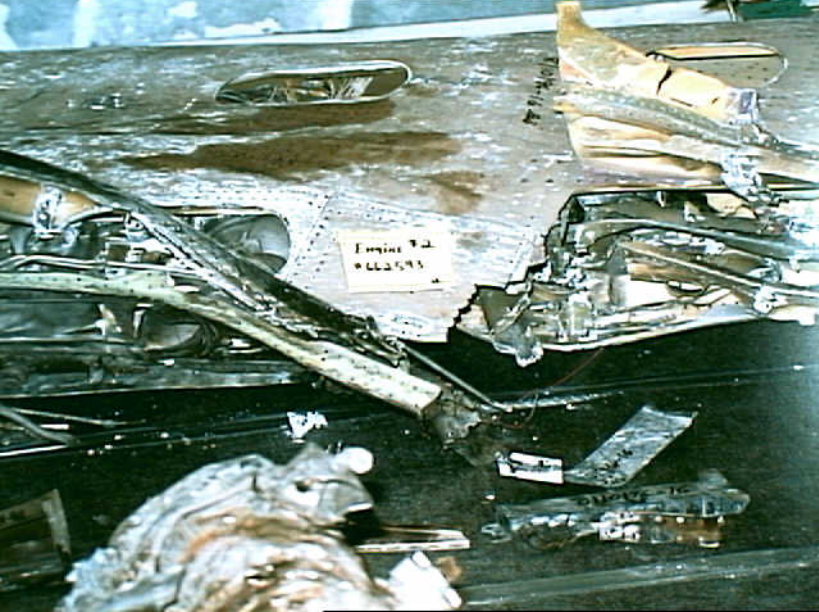
Powerplants 8 - Photo 16. Engine No. 2, pylon, left side.
