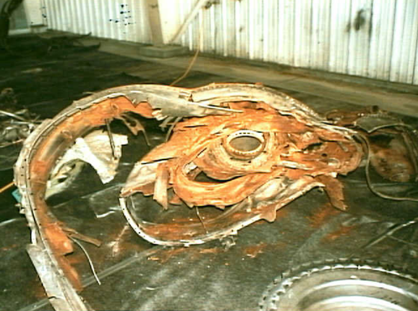
Powerplants 8 - Photo 15. Engine No. 1, turbine exhaust case (TEC) and No. 4 bearing housing
