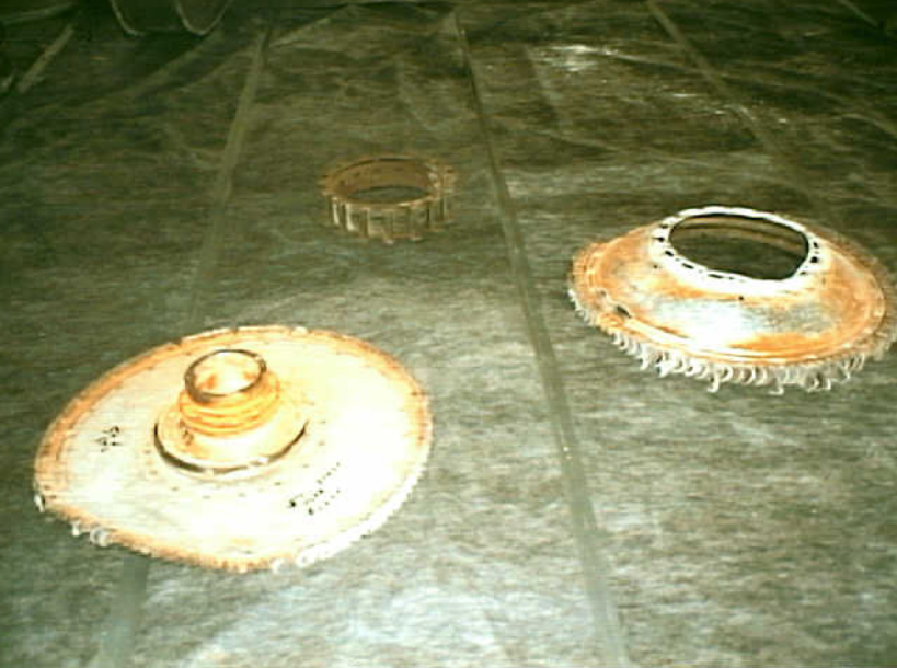
Powerplants 8 - Photo 14. Engine No. 1, 5th stage turbine hub and 6th stage turbine disk.
