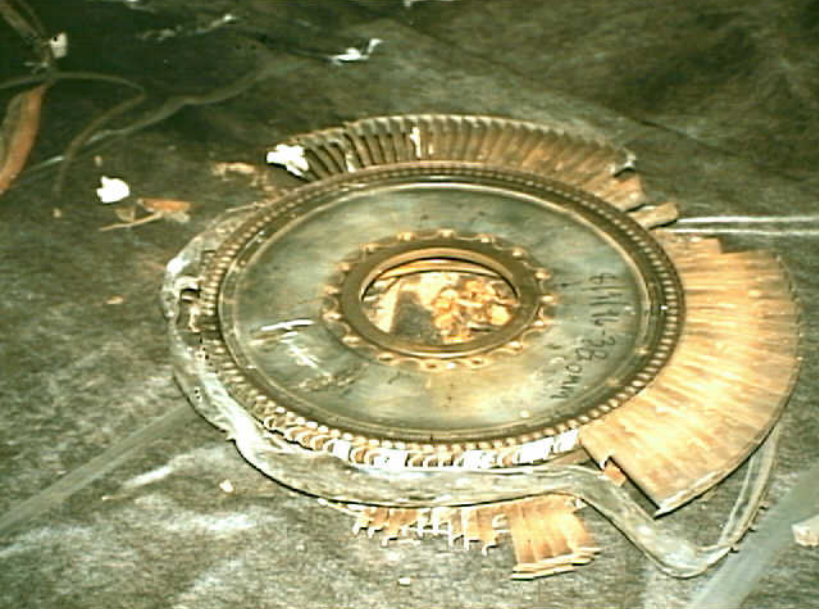
Powerplants 8 - Photo 13. Engine No. 1, LPT 3rd and 4th stage turbine disks and blades.
