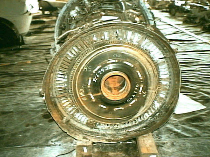
Powerplants 8 - Photo 12. Engine No. 1, rear of HPT showing 2nd stage disk, blades, and vanes.
