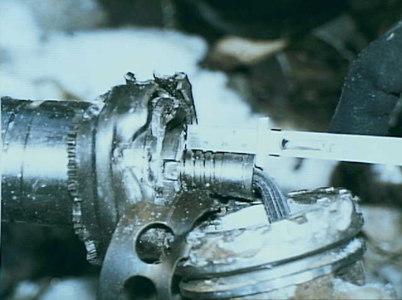
Powerplants 8 - Photo 10. Right propeller ball screw showing 1 \frac{7}{16} inch extension
