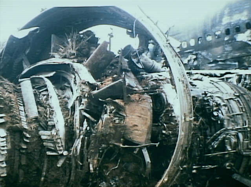
Powerplants 8 - Photo 10. No. 2 engine bottom, fan ring, and LPC
