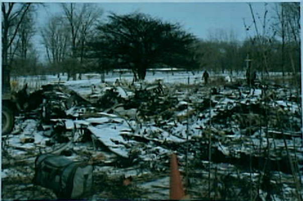
Powerplants 8 - Photo 1. View of wreckage showing center crater and left and right engines and propellers
