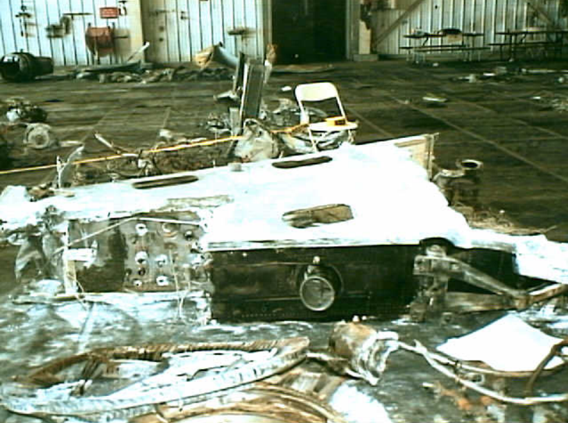
Powerplants 8 - Photo 1. Engine No. 1 pylon, left side.
