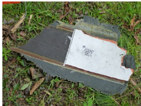
Figure 9. Inlet cowl outer barrel skin fragment
