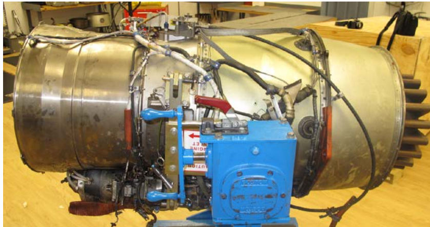
Photo 9- Left Hand Side of Engine with Airframe Components, Exhaust, and Inlet Cases Removed
