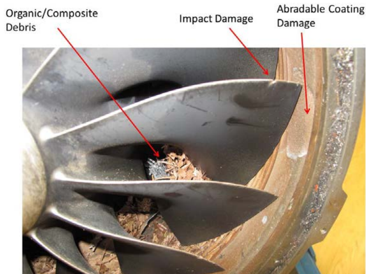
Photo 11- Compressor Inlet Fan Damage
