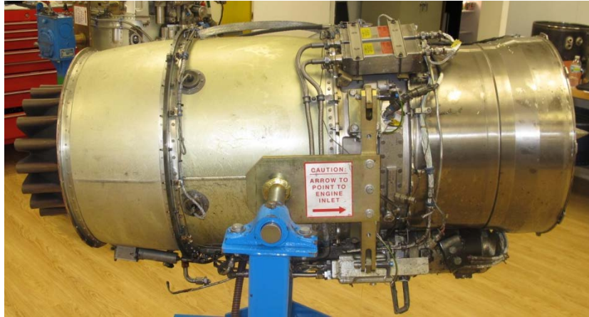
Photo 10- Right Hand Side of Engine with Airframe Components, Exhaust, and Inlet Cases Removed
