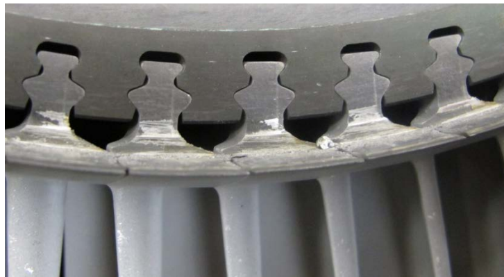
Photo 20- LPT 1 st Stage Blade Fir Tree Platform Rub Marks
