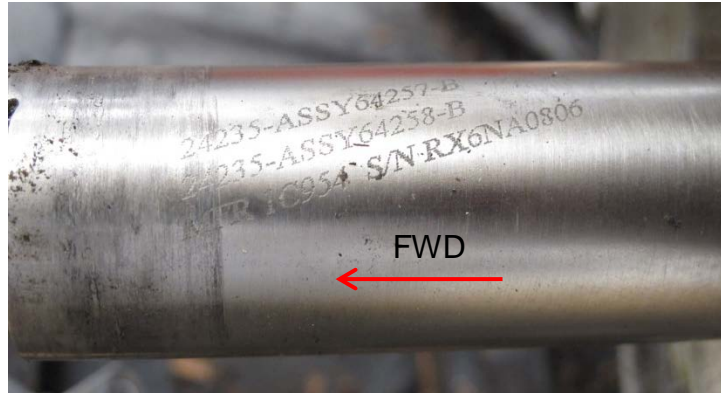
Photo 8- LPT Shaft Twisting (Part Etching Should Be Straight)
