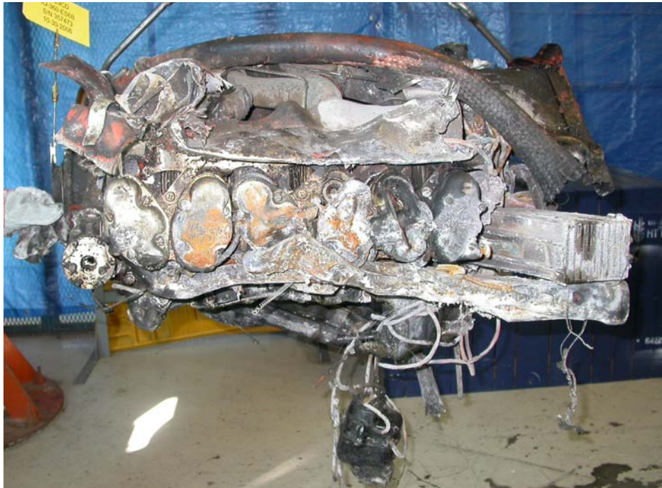
Figure 5. Crush and contact damage to LH side of engine
