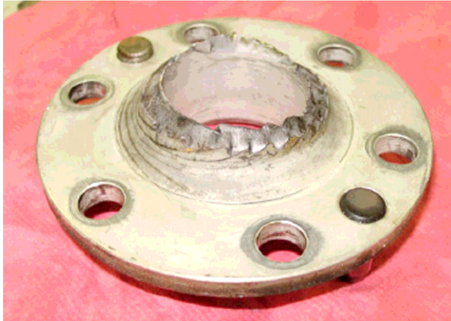
Figure 3. Propeller flange fracture
