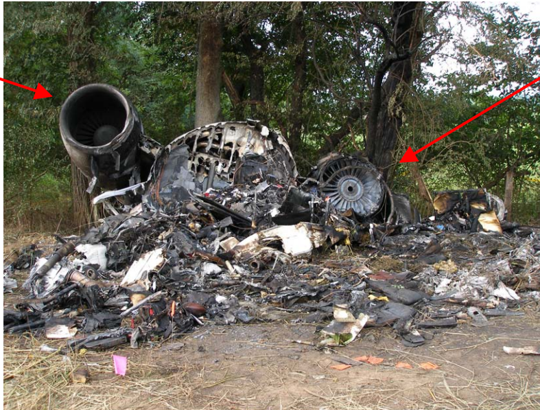
Figure 2 – Aft fuselage showing engines and pylons – Front view
