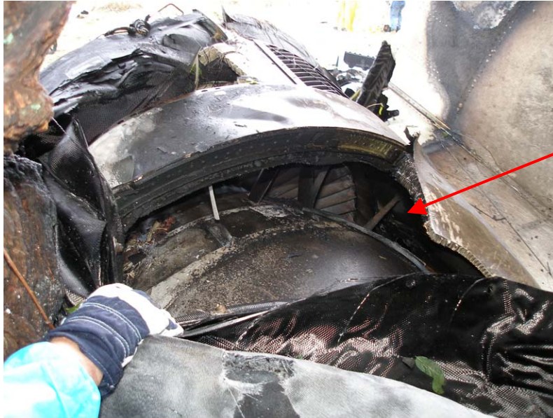
Figure 9 – Left-hand engine – Thrust reverser blocker doors stowed
