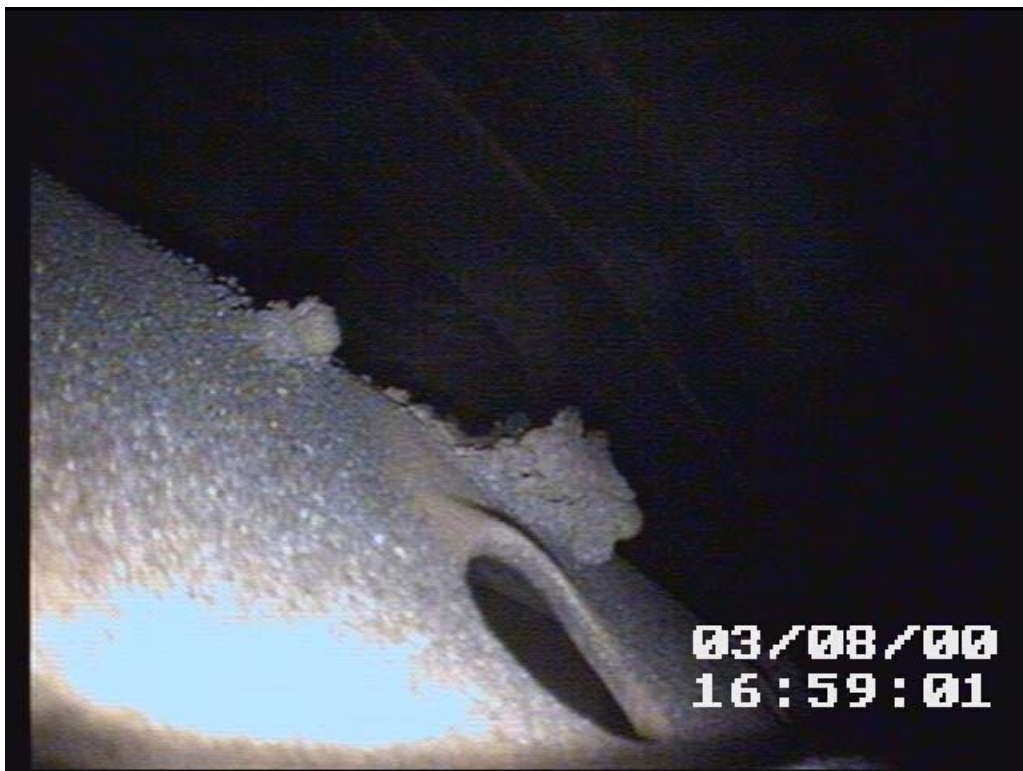
Photo 6: No. 2 engine combustion chamber with material deposits
