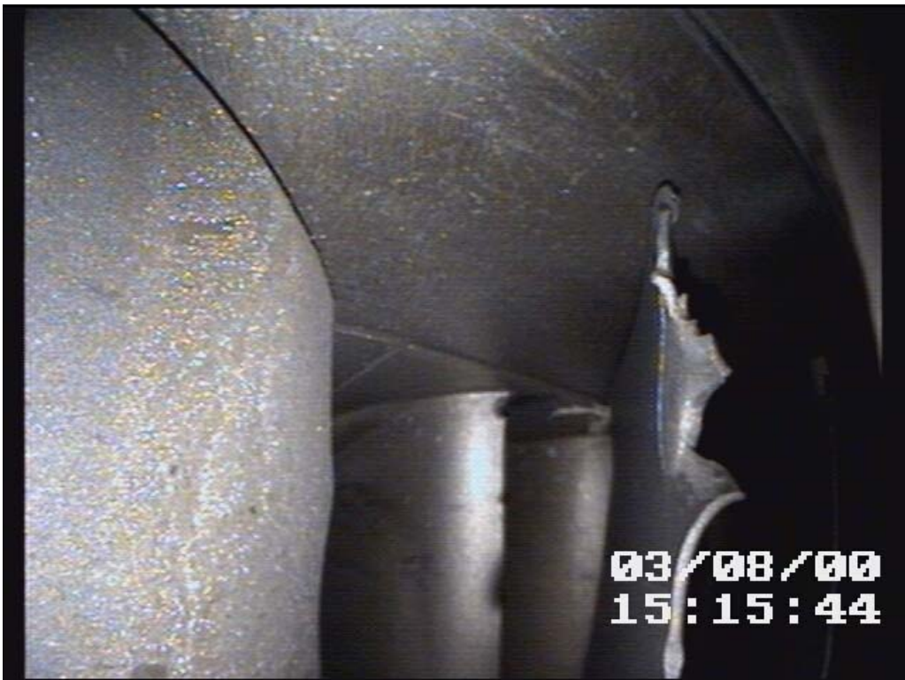
Photo 2: No. 1 engine compressor blade and vane damage
