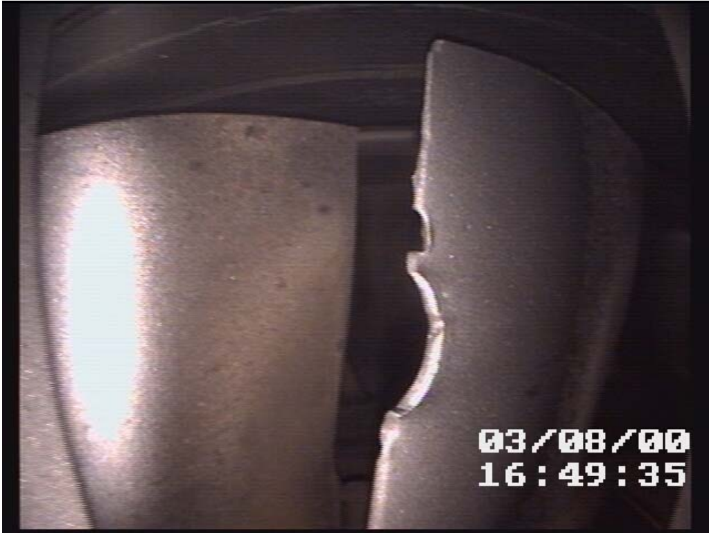
Photo 3: No. 2 engine compressor blade and vane damage
