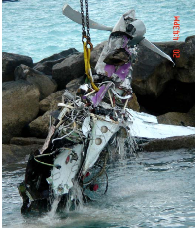
Figure 3. No. 2 engine recovered from Governor's Cut
