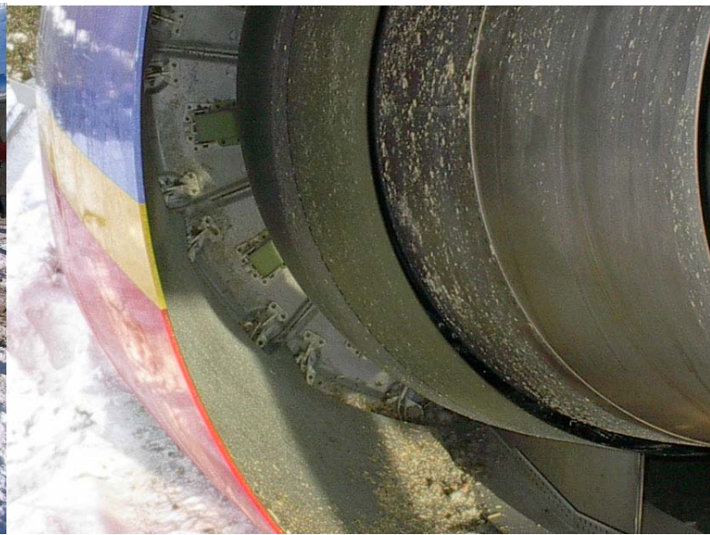
PHOTO 7: CLOSED BLOCKERS DOORS
