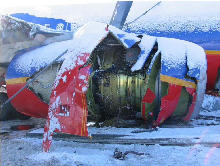
PHOTO 14: RIGHT HAND-COWL & TR DAMAGE
