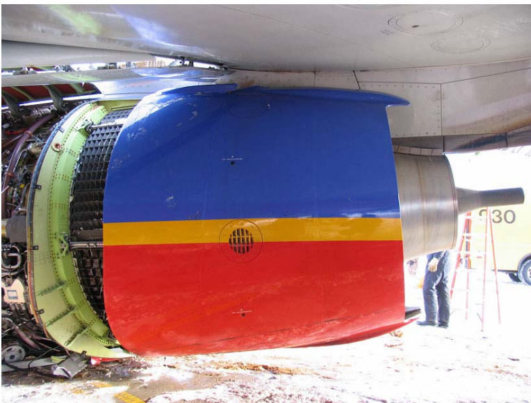
PHOTO 12: LEFT-HAND TR DEPLOYED
