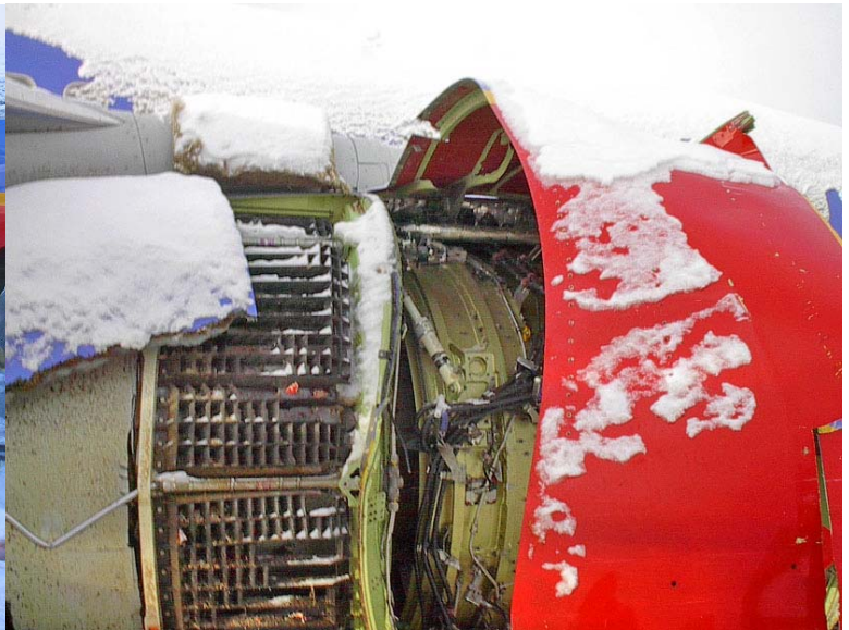
PHOTO 15: TORQUE BOX SEPERATED FRM FRAN FRAME
