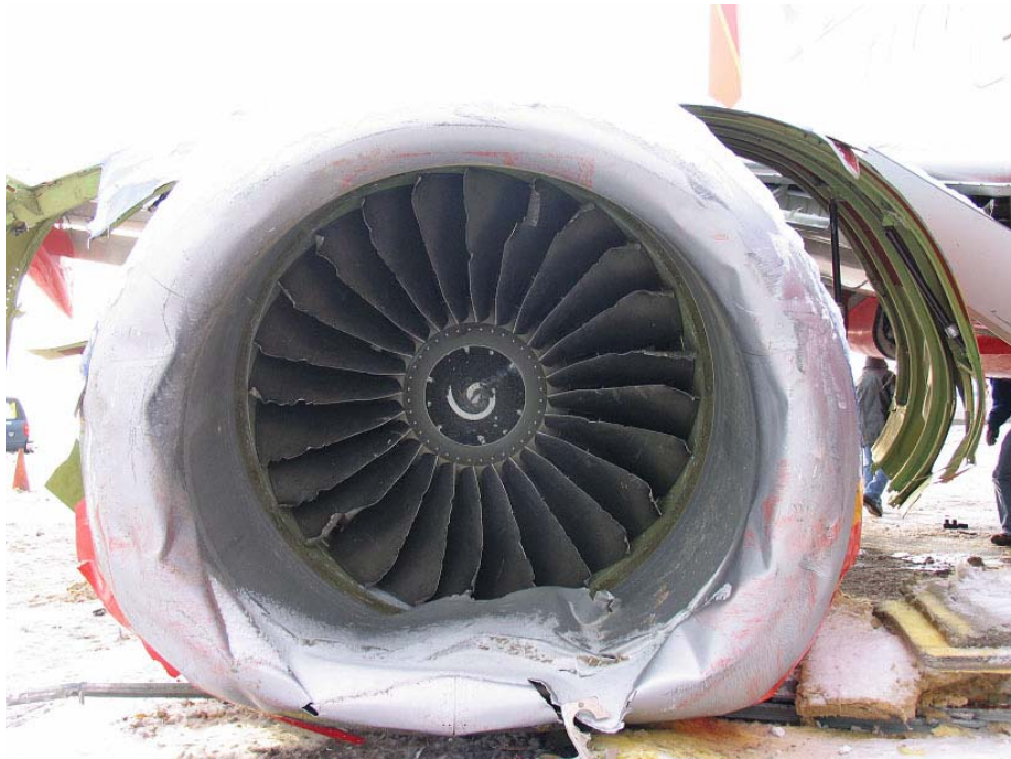
PHOTO 16: FAN SECTION AND INLET OF NO. 2 ENGINE
