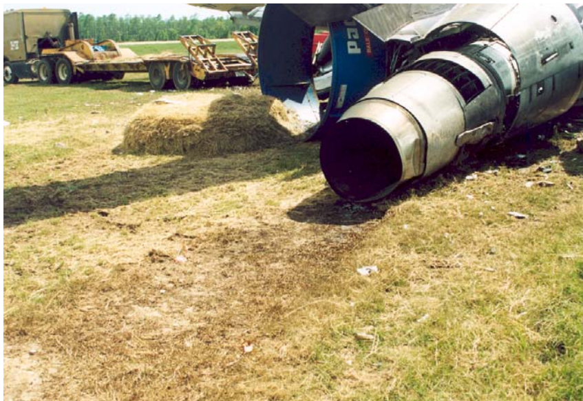
Photo 4: Area of scorched grass in back of No. 2 engine's exhaust
