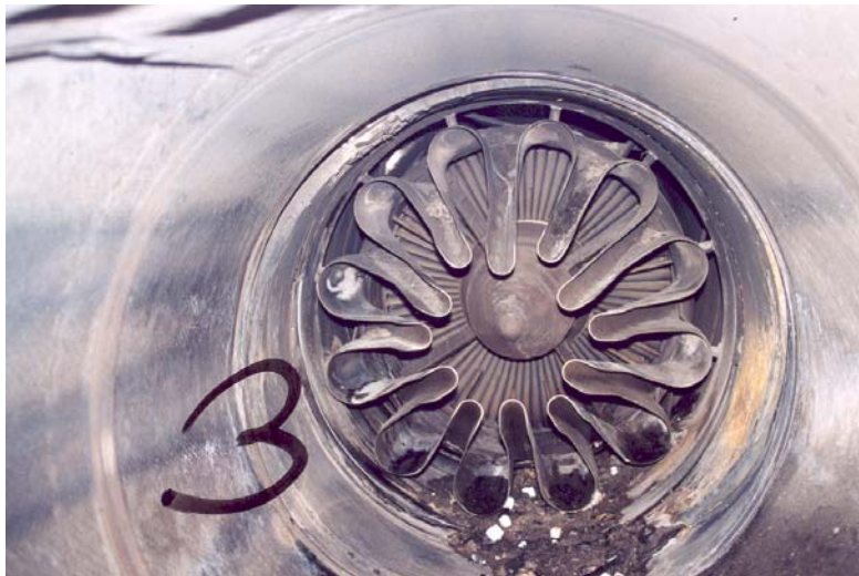
Photo 11: No. 3 engine's 4 th stage turbine blades showing no damage
