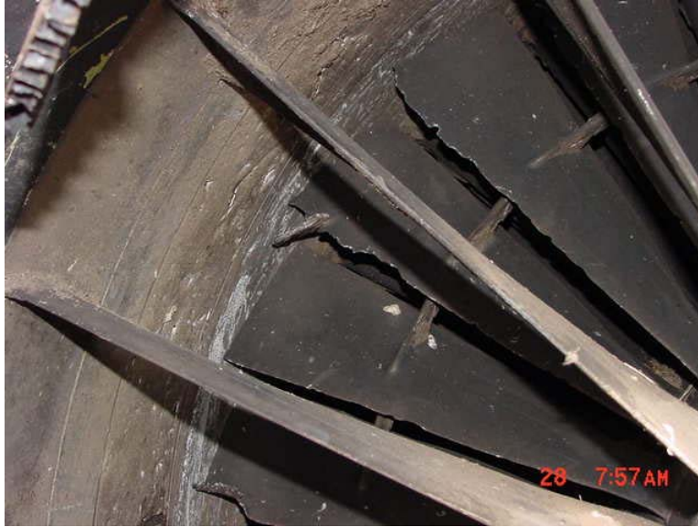
Photo 10. No. 3 engine's fan blades showing soft body impact damage and metallic object embedded into leading edge of one blade (FedEx)
