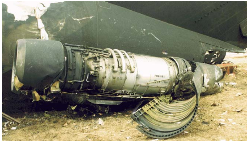
Photo 1: No. 1 engine with cowling removed
