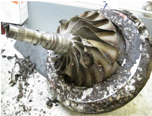
PHOTO 13: 1 ST -STG IMPELLER BLADE DAMAGE AND COMPRESSOR DIFFUSER PACKED WITH DIRT
