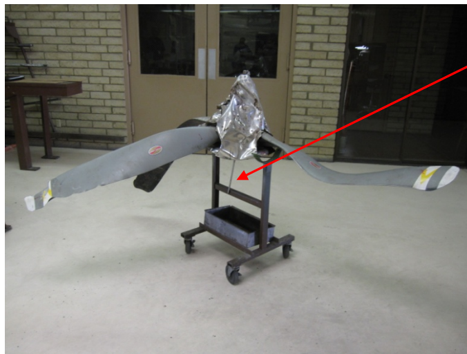
PHOTO 27: AS-RECEIVED PROPELLER WITH 'BETA' TUBE STILL INSTALLED
