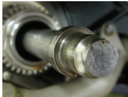
PHOTO 11: SHEARED COUPLING SHAFT
