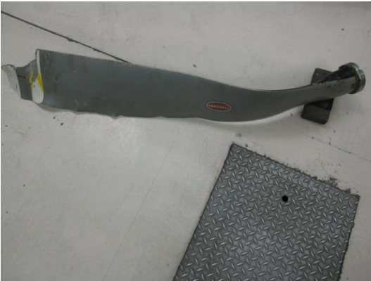
PHOTO 41: NO. 1 BLADE AIRFOIL DAMAGE
