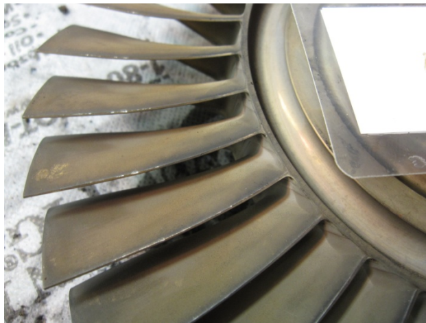
PHOTO 26: TRAILING EDGE IMPACT DAMAGE ON THE 3 RD -STAGE TURBINE ROTOR BLADES
