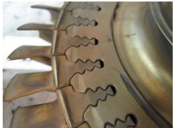
PHOTO 21: AFT INNER PLATFORMS SCORING
