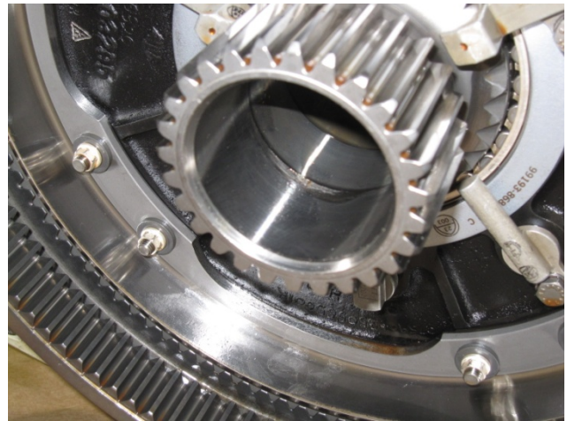
PHOTO 9: SUN GEAR INNER LOCALIZED SCORING
