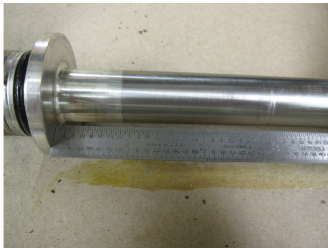
PHOTO 40: PITCH CHANGE ROD WITH CIRCUMFERENTIAL SCORE MARK
