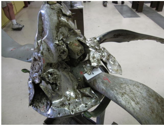
PHOTO 28: SPINNER DOME DAMAGE WITH THE NO. 4 COUNTERWEIGHT PUNCTURED THROUGH THE SKIN
