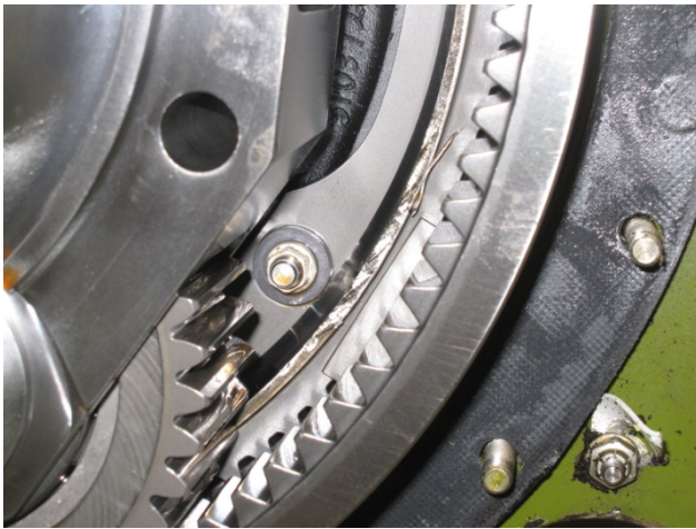
PHOTO 8: RING GEAR BUMPER LOCALIZED SCORING
