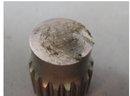
PHOTO 12: SHEARED COUPLING SHAFT
