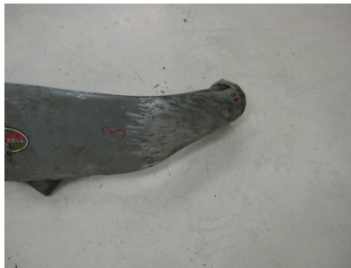
PHOTO 45: AIRFOIL SPANWISE SCRATCHES
