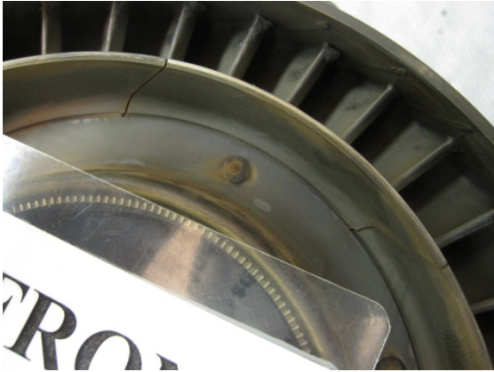
PHOTO 22: LOCALIZED SCORING OF INNER VANE SUPPORT
