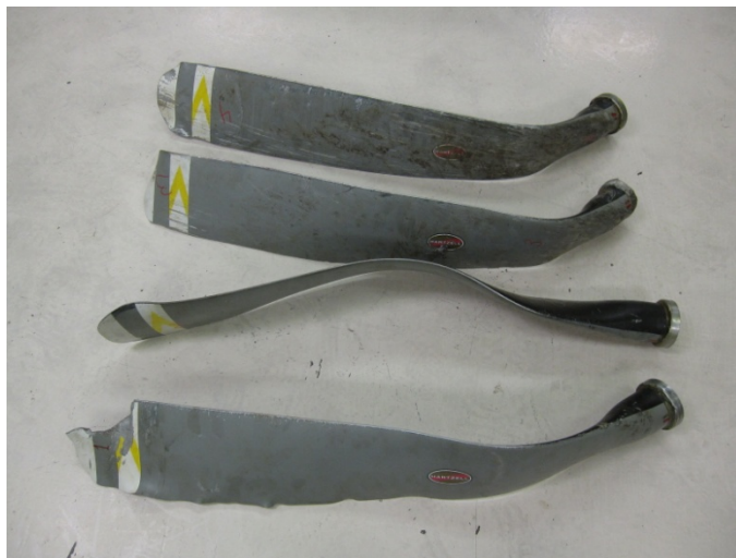
PHOTO 47: NO. 4 PROPELLER DAMAGE (TOP OF PICTURE) SIDE BY SIDE WITH THE OTHER BLADES
