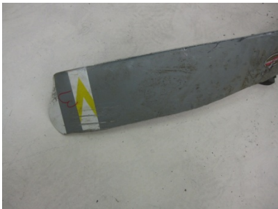
PHOTO 44: NO. 3 BLADE AIRFOIL TIP CURLED
