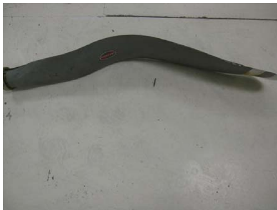
PHOTO 43: NO. 2 BLADE AIRFOIL DAMAGE
