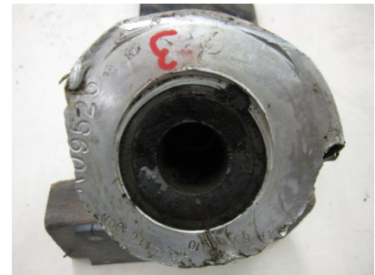
PHOTO 46: RETENTION SHOULDER DAMAGE
