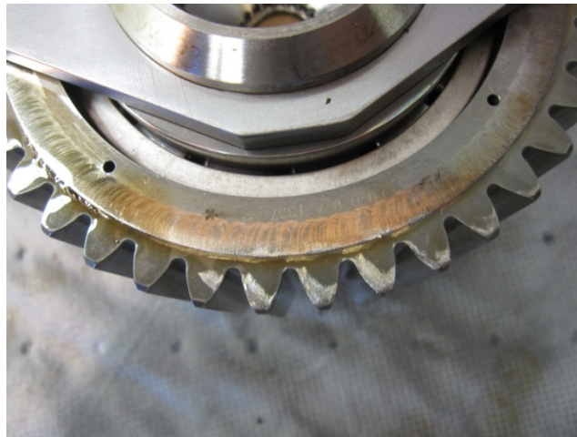
PHOTO 7: PLANETARY GEAR TEETH WITH CONTACT SCORING
