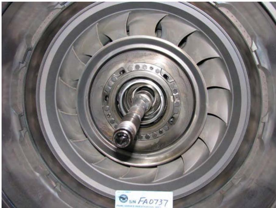
Figure 17. Inter-stage turbine vane ring
