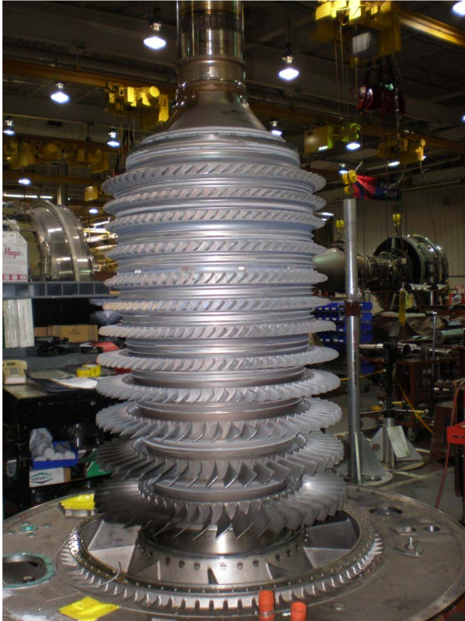
Photo 17: HPC rotor showing all of the blades were in place
