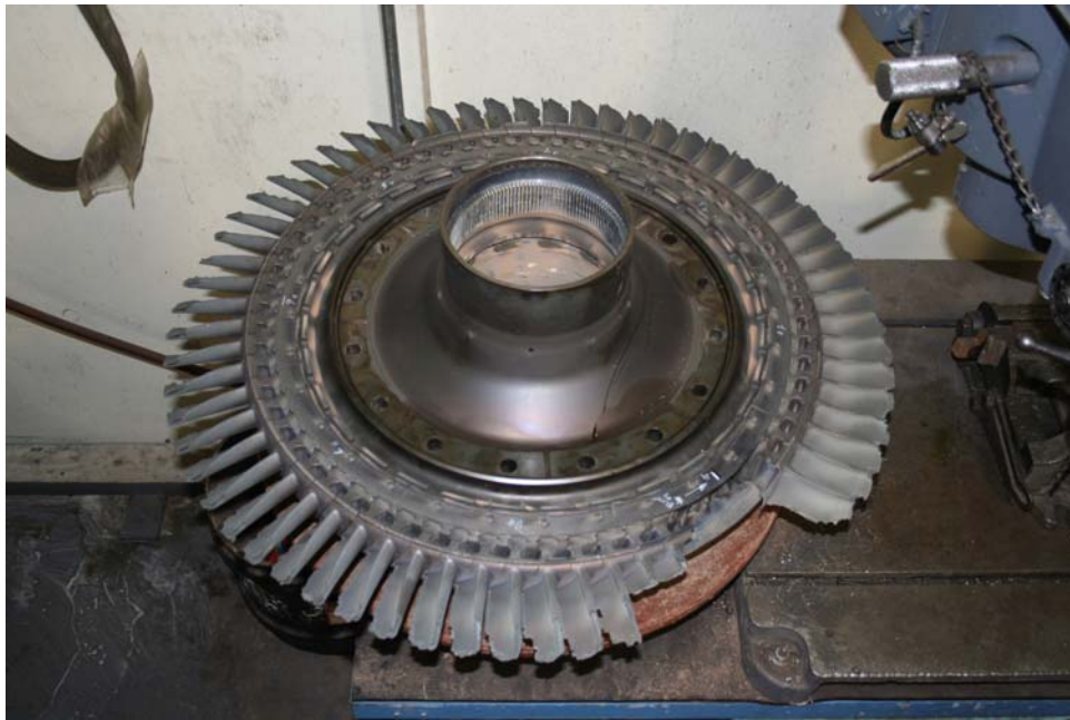
Photo 5: 2nd stage hub with 2nd stage turbine blades showing missing blades, blades fractured near platform, and remaining blades damaged (P&W)
