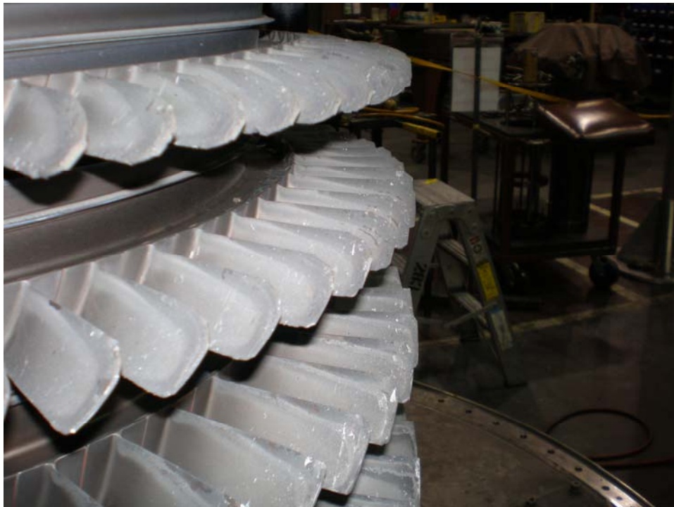
Photo 19: Burned compressor blade tips at rear of compressor
