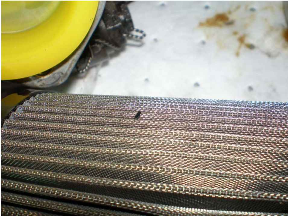
Photo 27: Debris in oil filter screen
