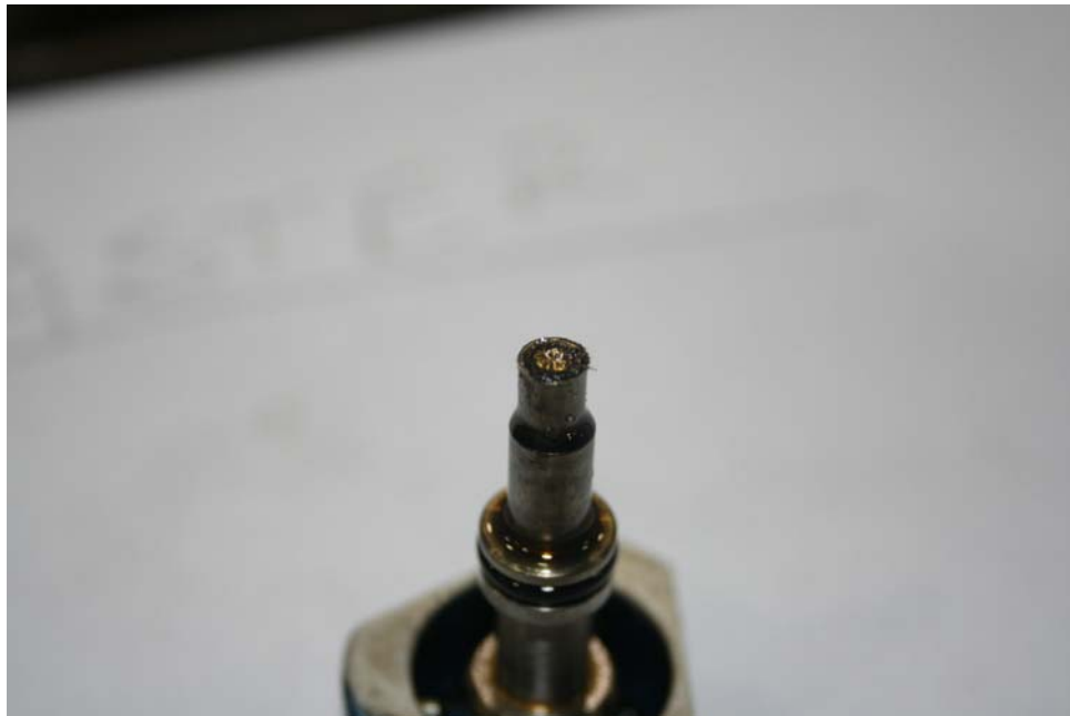
Photo 29: Metallic material on master MCD (P&W)
