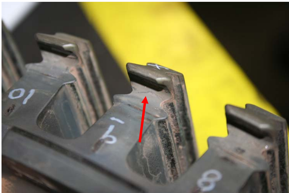
Photo 4: Close up of lug No. 9 with arrow showing crack (P&W)
