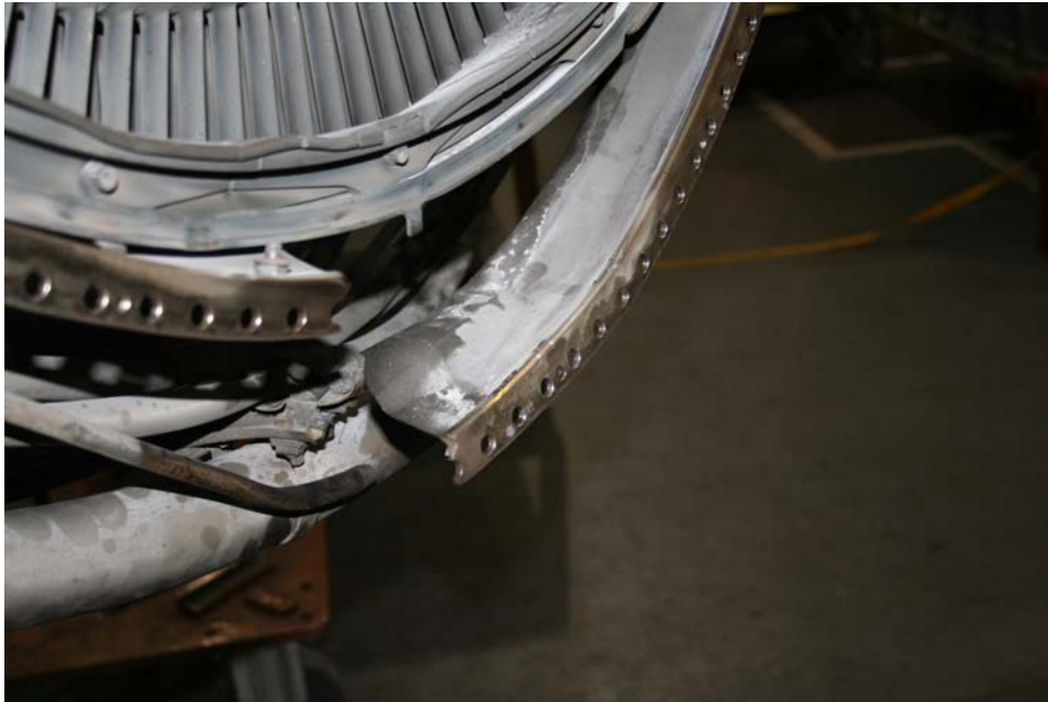
Photo 21: View of LPT case showing displacement of fractured front flange (P&W)
