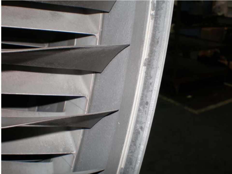
Photo 16: 5th stage compressor blades with groove worn in rub strip
