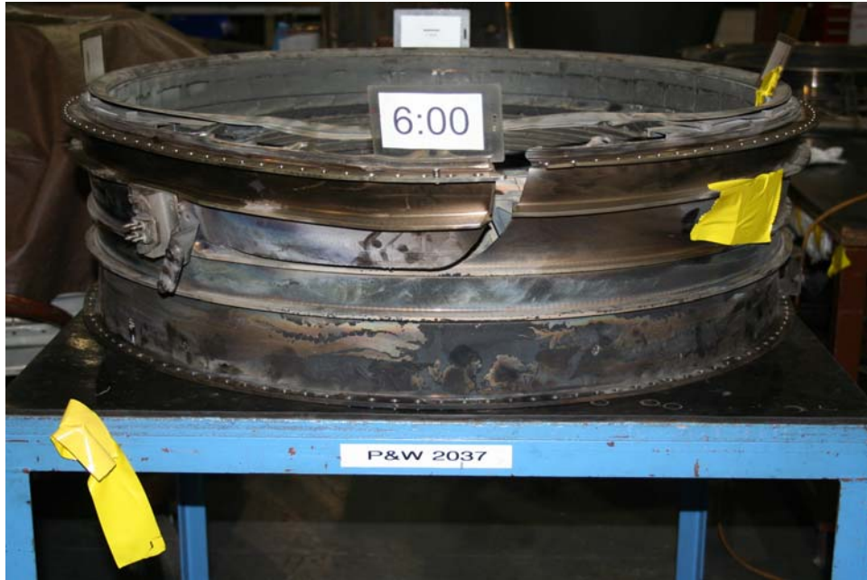
Photo 9: View of tab of displaced material on ruptured HPT case (P&W)
