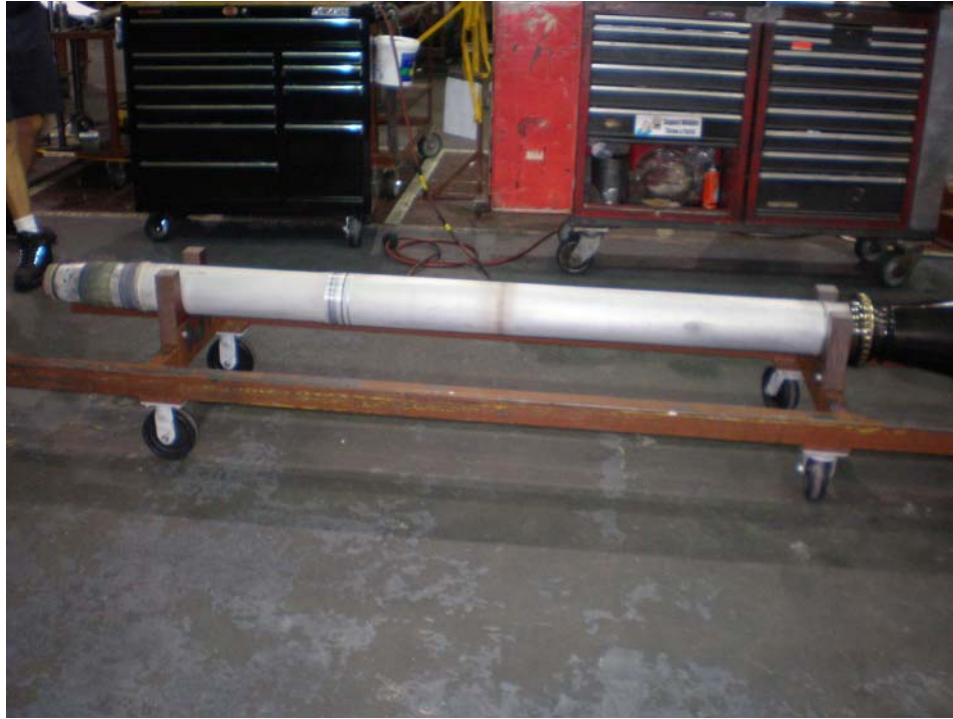
Photo 22: LPT shaft showing various circumferential rub marks
