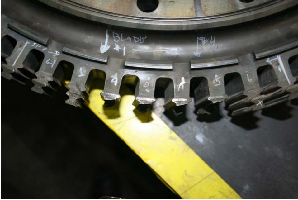
Photo 1: Close up of 2nd stage turbine hub showing fractured lugs Nos. 2 through 5 (P&W)
