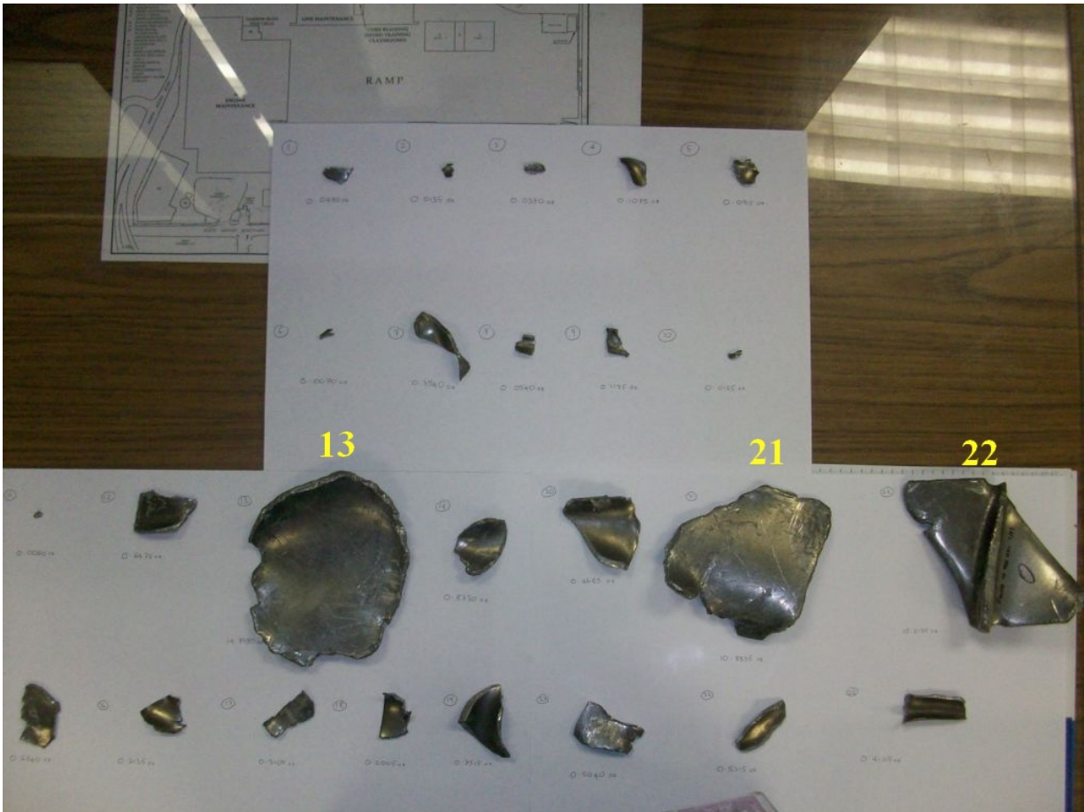
PHOTO 25: COLLECTED FAN BLADE FRAGMENTS FROM INLET COWL AND THRUST REVERSER (COURTESY OF UNITED AIRLINES)
