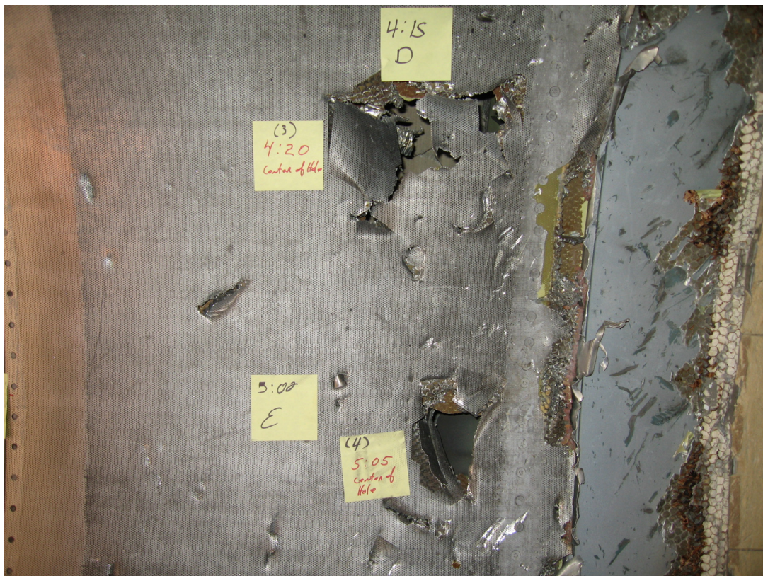
PHOTO 7: INLET COWL INNER BARREL DAMAGE - LOCATIONS 3 AND 4
