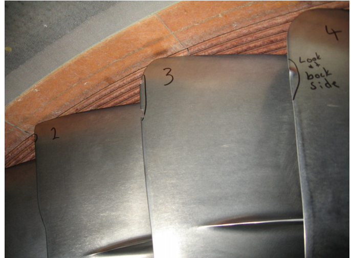
PHOTO 24: NO. 2 ENGINE FAN BLADE NO. 3 & 4 DAMAGE
