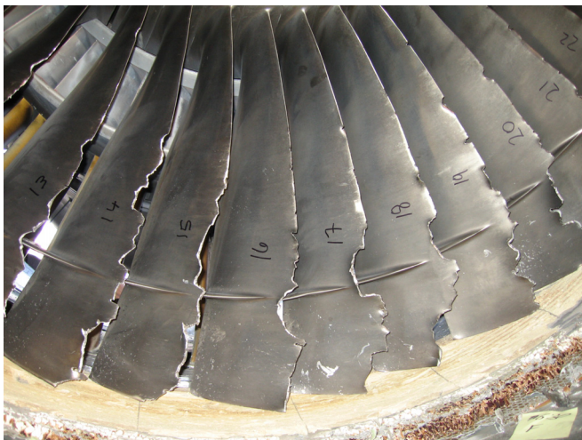
PHOTO 16: HARD-BODY FAN BLADE DAMAGE
