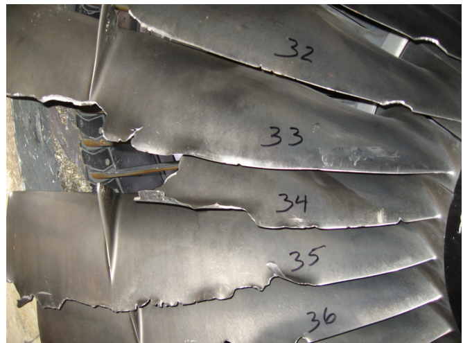
PHOTO 17: SOFT-BODY FAN BLADE DAMAGE
