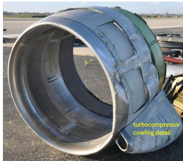
Figure 6. No. 2 engine inlet cowl
