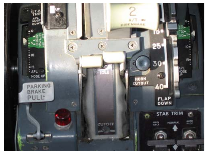
PHOTO 23: FUEL START LEVER POSITION
