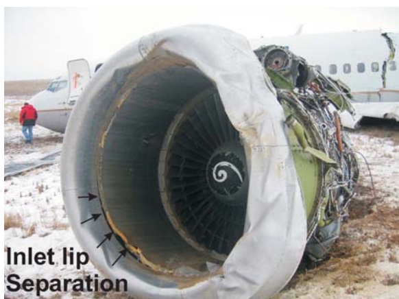
PHOTO 7: INLET LIP SEPARATION
