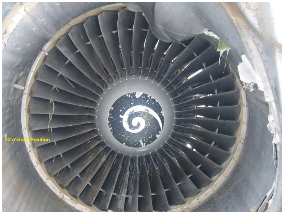
PHOTO 9: NO. 1 ENGINE FAN BLADE DAMAGE
