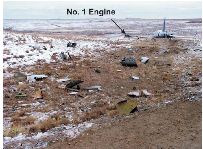
PHOTO 6: DEBRIS FIELD ALONG WRECKAGE PATH
