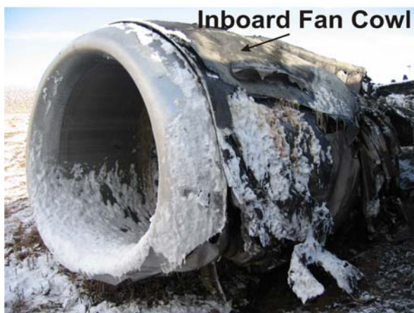
PHOTO 13: COWL FIRE DAMAGE INBOARD SIDE
