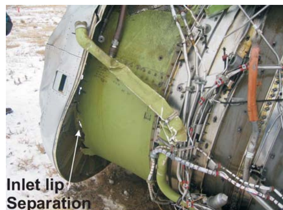
PHOTO 8: INLET LIP SEPARATION
