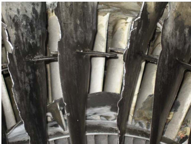
PHOTO 19: HARD BODY DAMAGE AND FAN BLADE FRAGMENT RESTING IN FRONT OF THE OGVs
