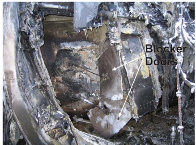
PHOTO 16: BLOCKER DOORS DEPLOYED
