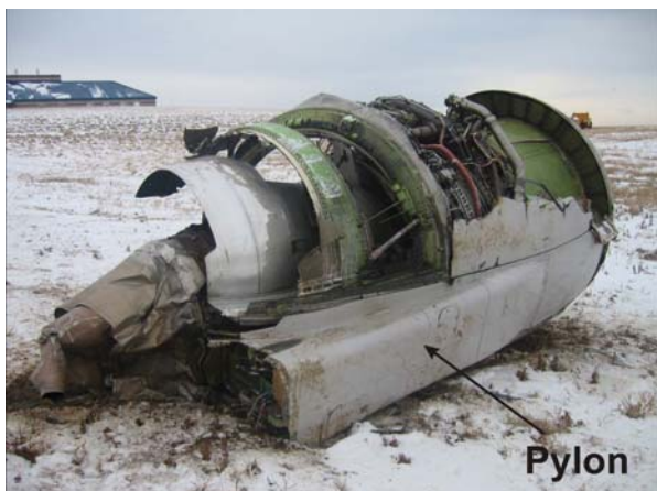
PHOTO 3: TOP OF ENGINE – PYLON ATTACHED
