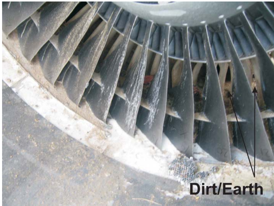
PHOTO 10: DIRT AND EARTH DEBRIS IN THE FAN AND BOOSTER SECTION
