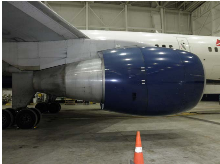
Photo No. 5: View of the right side of the engine with the nacelles in place showing no damage or sooting.
