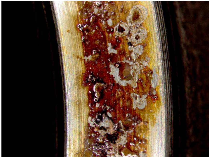
Photo No. 8: Close up view of FMV sleeve showing brown substance on chamfer. (Hamilton Sundstrand)
