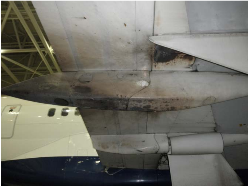
Photo No. 3: Right (outboard) side of the inboard flap track fairing showing damage on rear two-thirds of the rear fairing.
