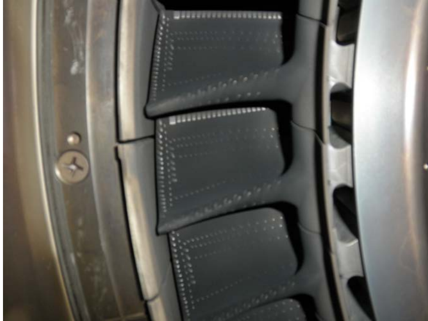
Photo No. 15: Close-up view of the 1st stage turbine blades showing the dark discoloration on the airfoil surface.
