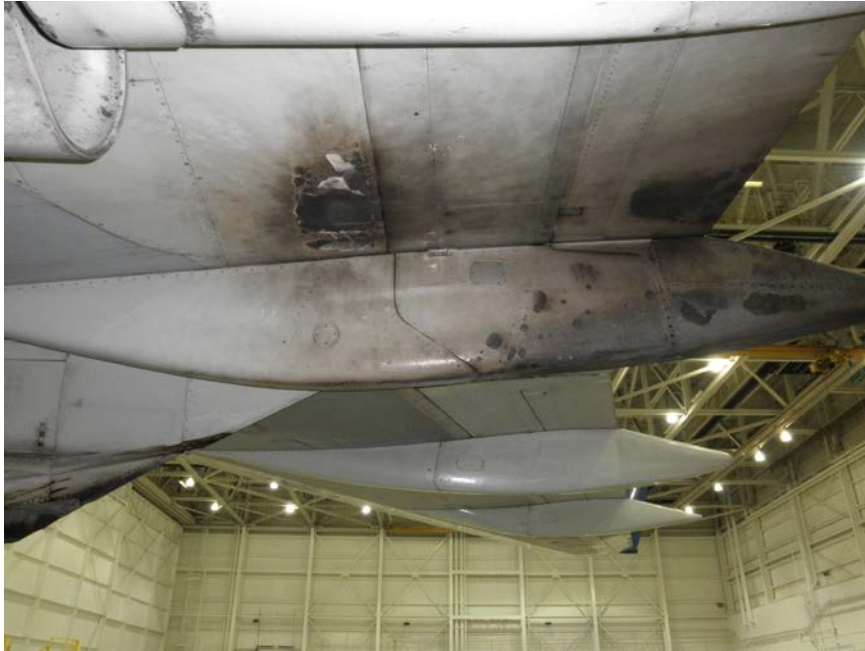
Photo No. 2: Left (inboard) side of the inboard flap track fairing showing damage on rear two-thirds of the rear fairing.
