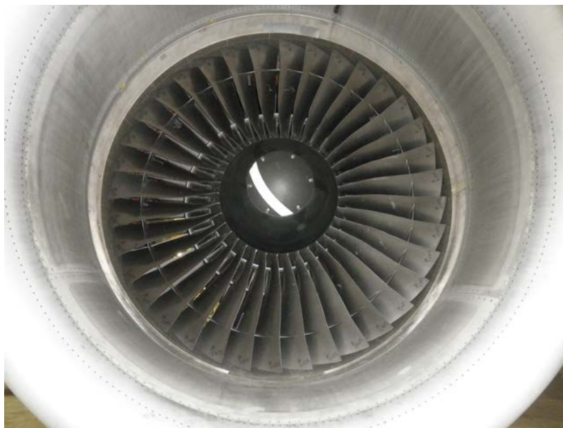
Photo No. 6: View of the front of the engine showing all of the fan blades were in place and undamaged.
