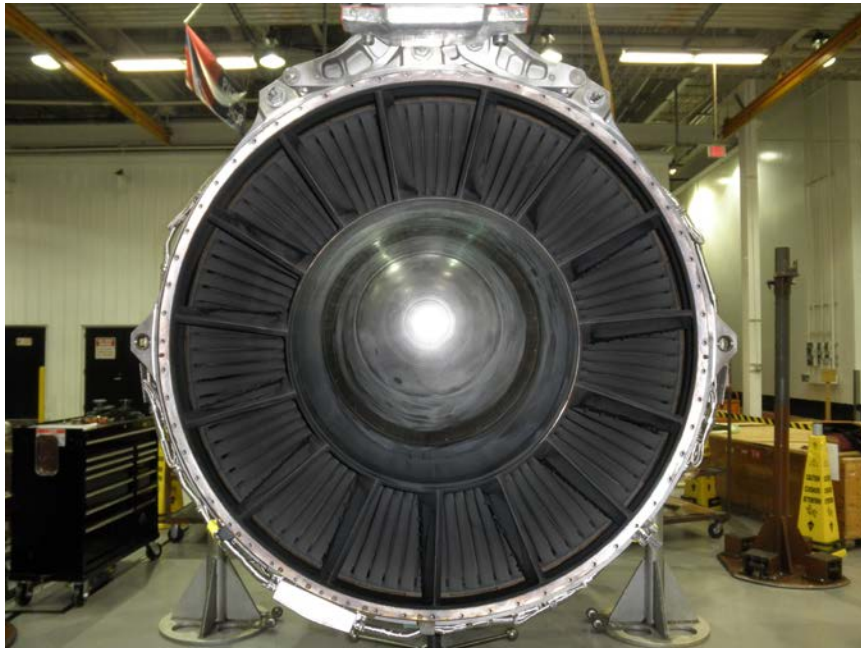
Photo No. 18: View of the 7th stage turbine blades showing dark discoloration.
