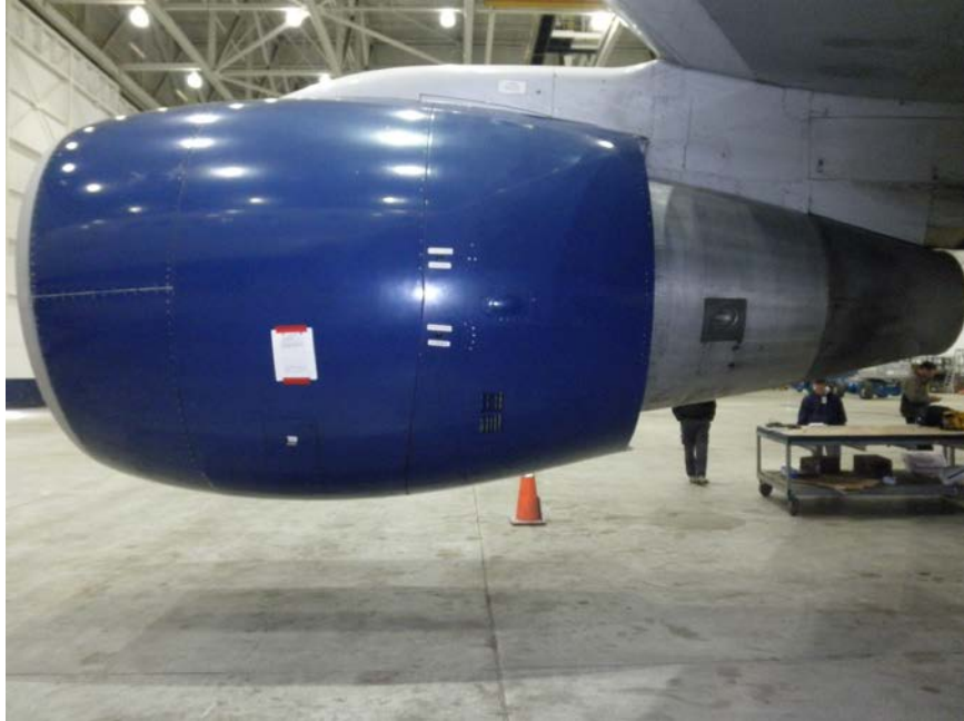
Photo No. 4: View of the left side of the engine with the nacelles in place showing no damage or sooting.
