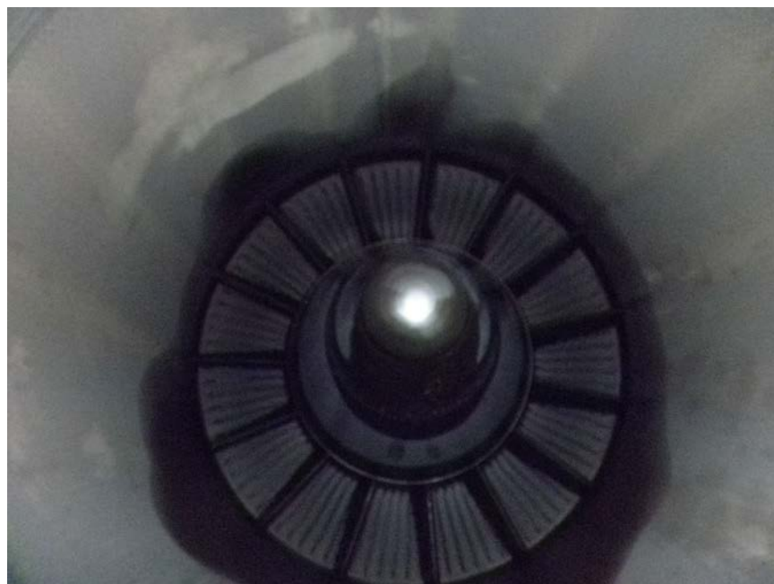
Photo No. 7: View of the rear of the engine showing all of the 7th stage turbine blades were in place and undamaged.
