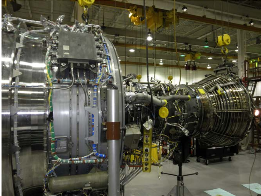
Photo No. 12: View of the left side of the engine showing no fire damage or sooting.
