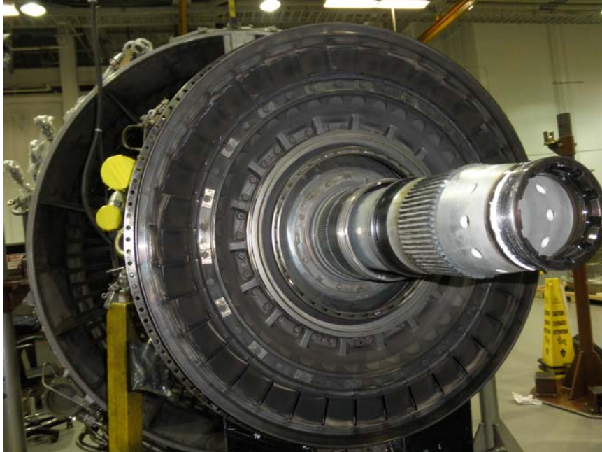
Photo No. 16: View of the 1st stage turbine vanes showing they were all in place and had a dark discoloration.
