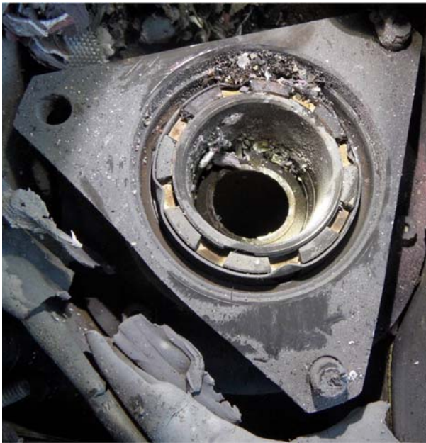
Figure 6. Power takeoff flange and aft fracture surface of freewheel shaft
