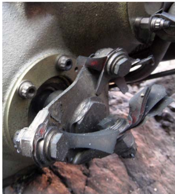
Figure 7. Tail rotor drive flange coupling damage
