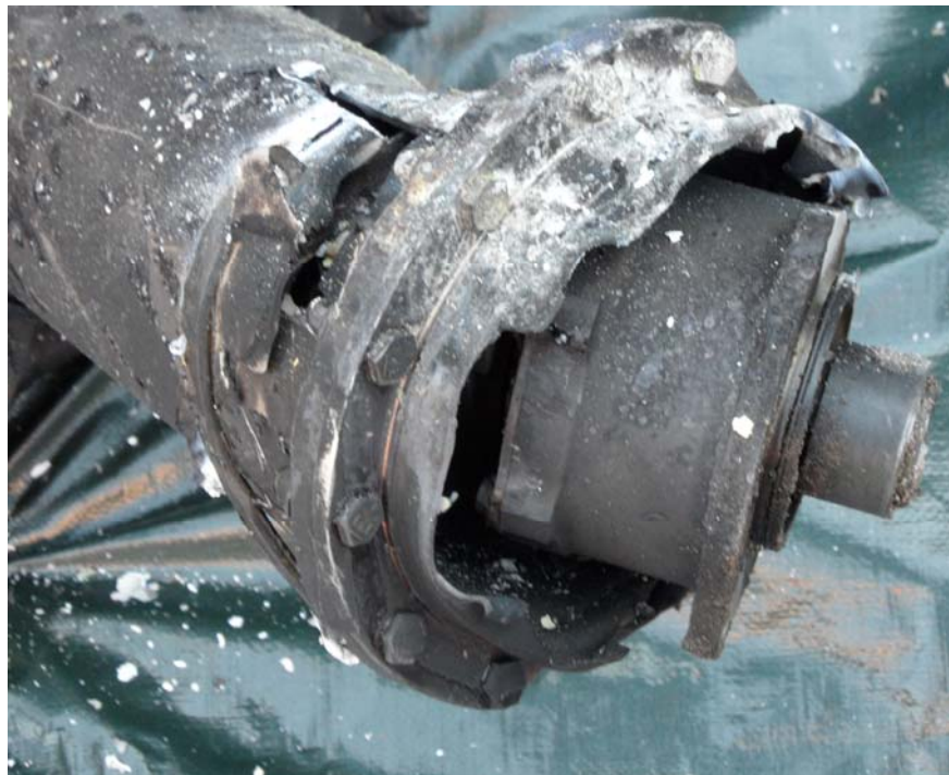
Figure 10. Freewheel unit with forward section of freewheel shaft in helicopter main gearbox drive shaft housing
