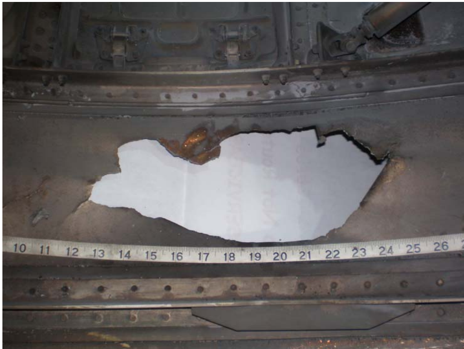
Photo 31: Hole in left core cowl
