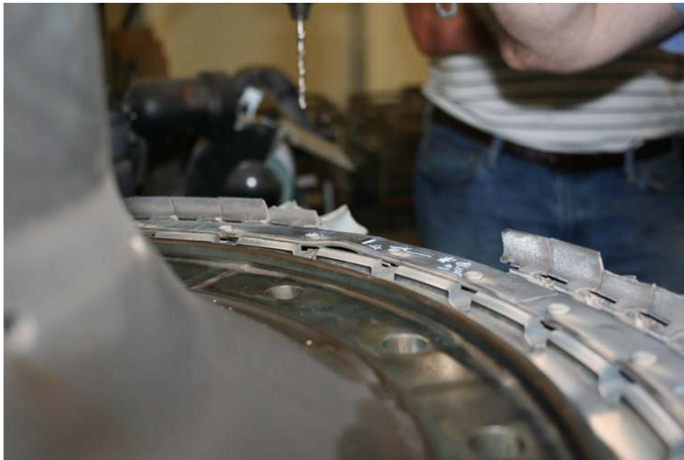
Photo 8: Front 2nd stage turbine blade retaining plate that was buckled (P&W)
