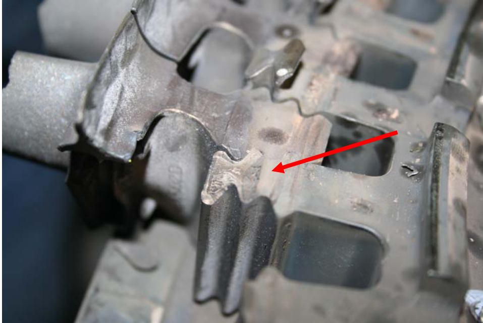
Photo 2: Close up of lug No. 1 with arrow pointing to the dark-colored, elliptical-shaped fracture surface feature (P&W)
