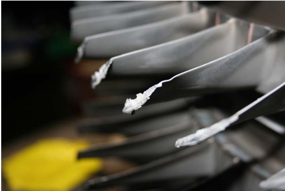
Photo 18: 8 th stage compressor blades showing displaced material on the tips (P&W)
