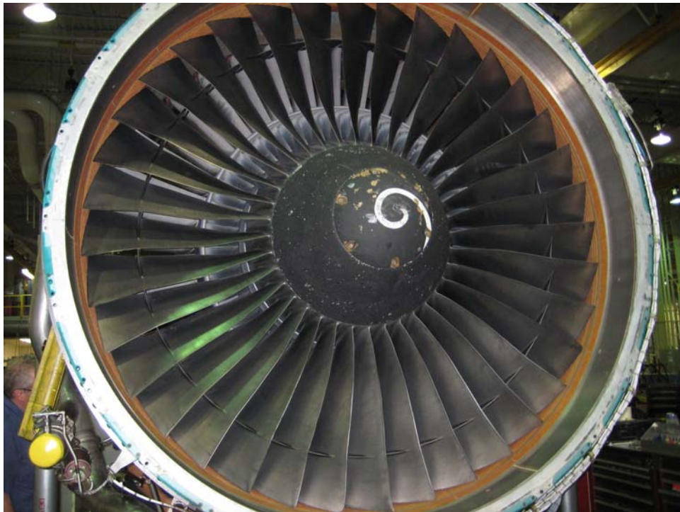
Photo 15: Fan blades all in place and undamaged (Delta)
