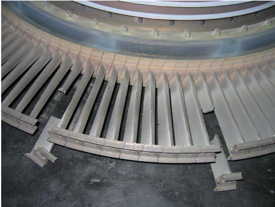
Photo 23: 3rd stage turbine blades showing random broken blades (Boeing)
