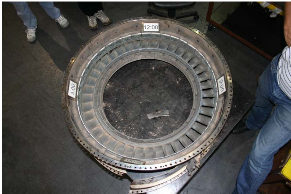
Photo 13: 2nd stage turbine vanes all in place in the HPT case (P&W)
