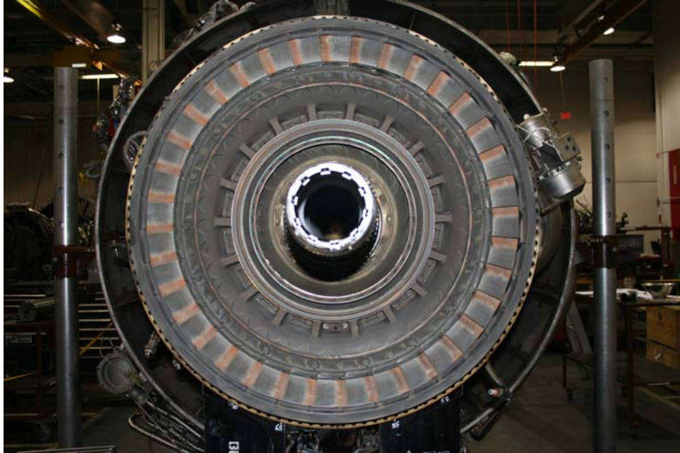
Photo 12: 1st stage turbine vanes all in place (P&W)
