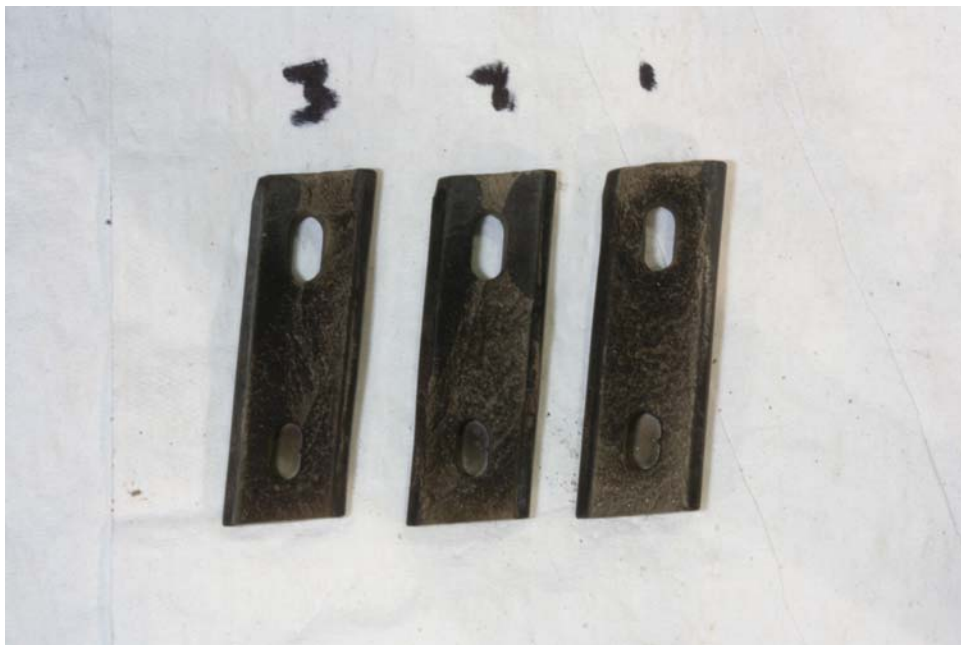
Photo 6: Close up of fractured 2nd stage turbine blade root ends (P&W)
