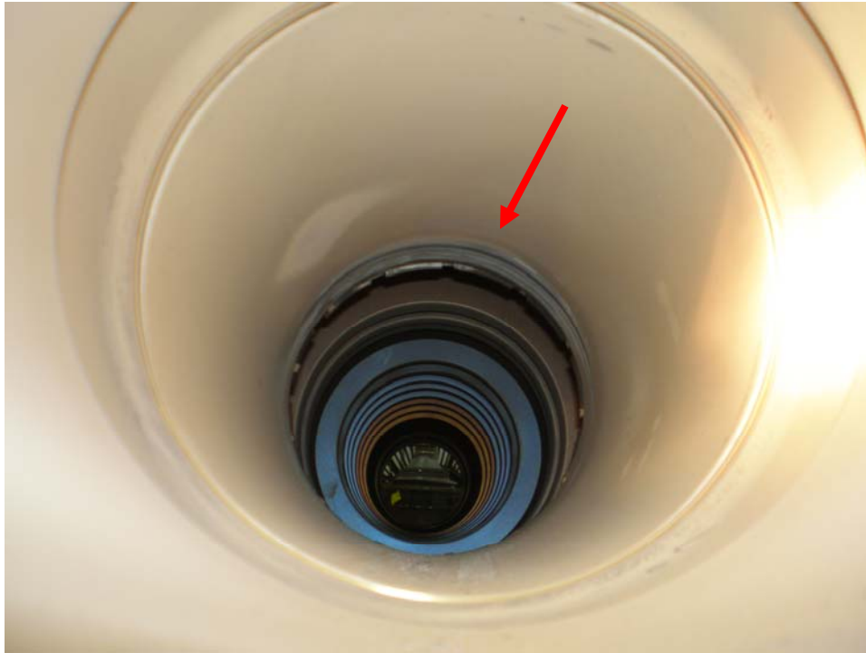
Photo 10: Inside of HPT shaft with arrow showing rub mark
