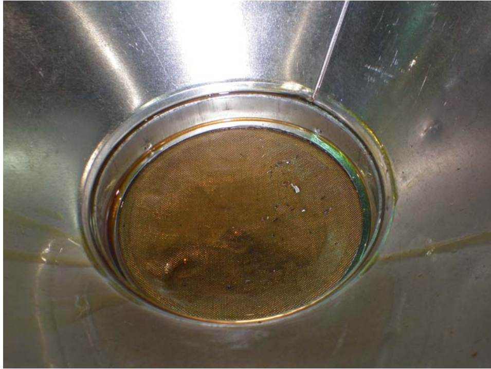
Photo 26: Metal debris in screen from oil drained from engine oil tank
