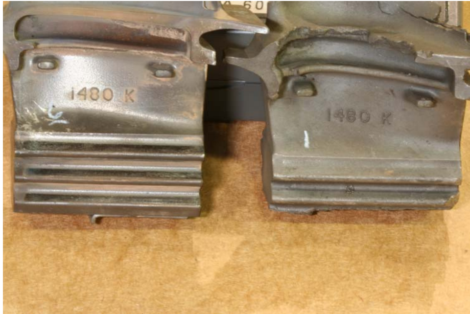
Photo 7: 2 nd stage turbine blades Nos. 1 and 6 showing different wear patterns on root fir trees (P&W)
