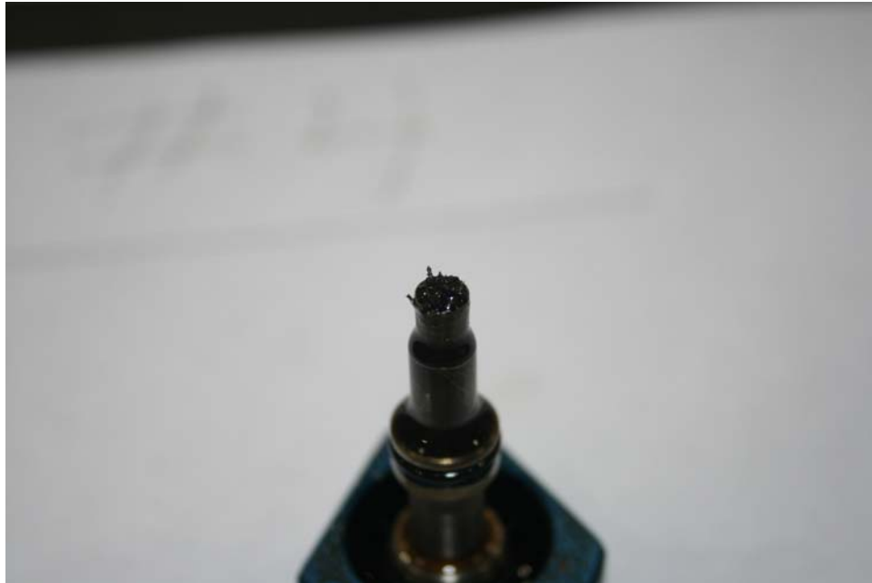
Photo 28: Metallic material on No. 4 bearing MCD (P&W)
