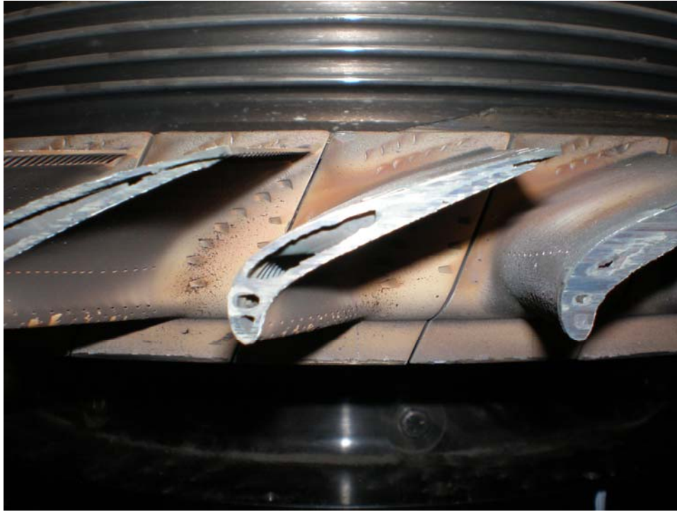
Photo 11: Close up of 1st stage turbine blade tips showing rub into internal cavity
