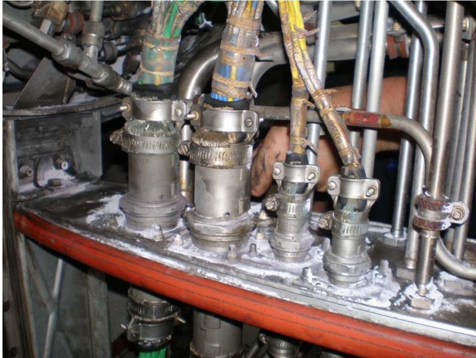
Photo 14: Close up of bifurcation panel showing dry chemical fire extinguishing agent
