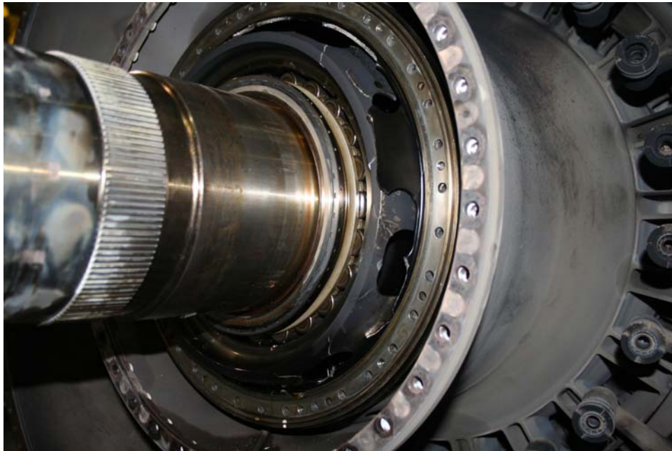
Photo 30: No. 4 bearing showing roller ends and broken housing (P&W)
