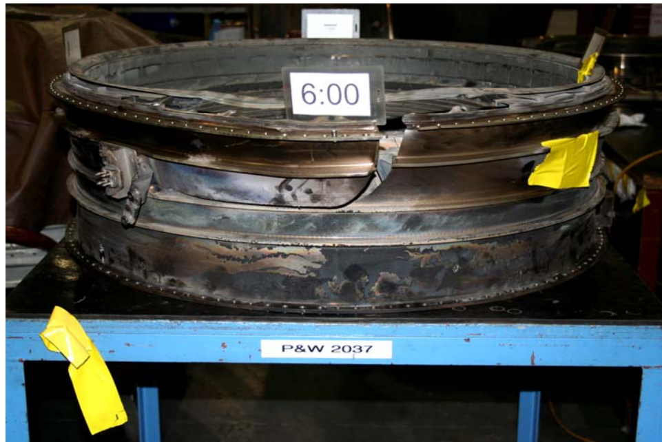
Photo 9: View of tab of displace material on ruptured HPT case (P&W)
