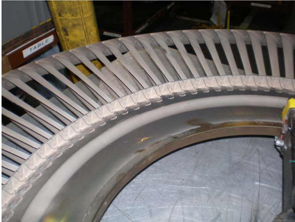
Photo 25: 5th stage turbine blades
