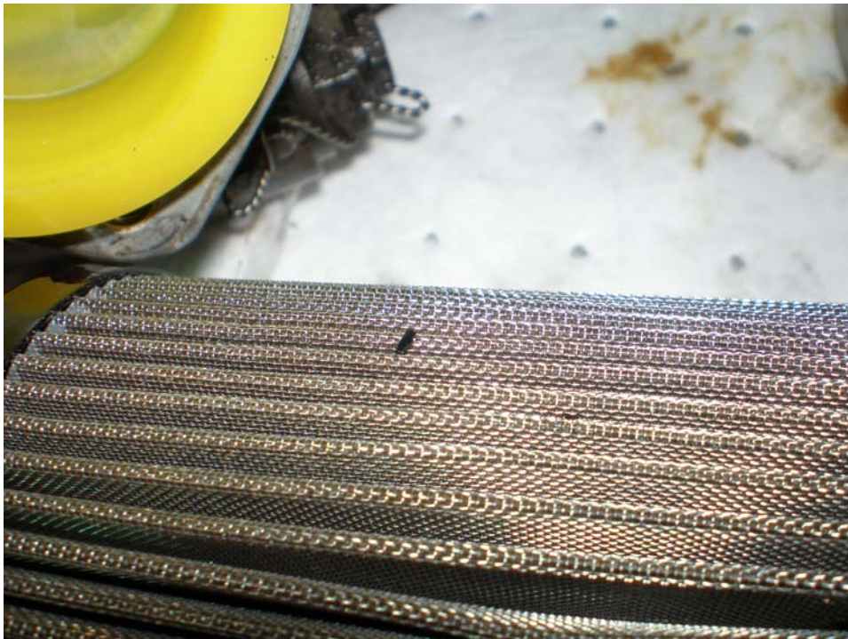
Photo 27: Debris in oil filter screen
