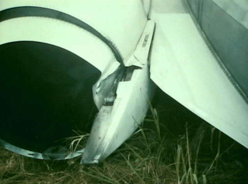
Powerplants 8 - Exhibit No. 8B - Photo 5. Rear view of No. 1 engine thrust reverser showing damage. (APA photo)
