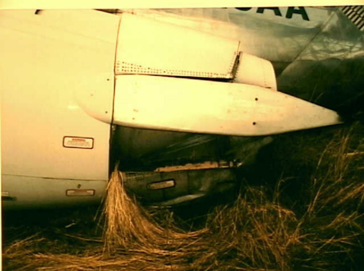
Powerplants 8 - Exhibit No. 8B - Photo 4. Side view of No. 1 engine thrust reverser showing partial deployment.
