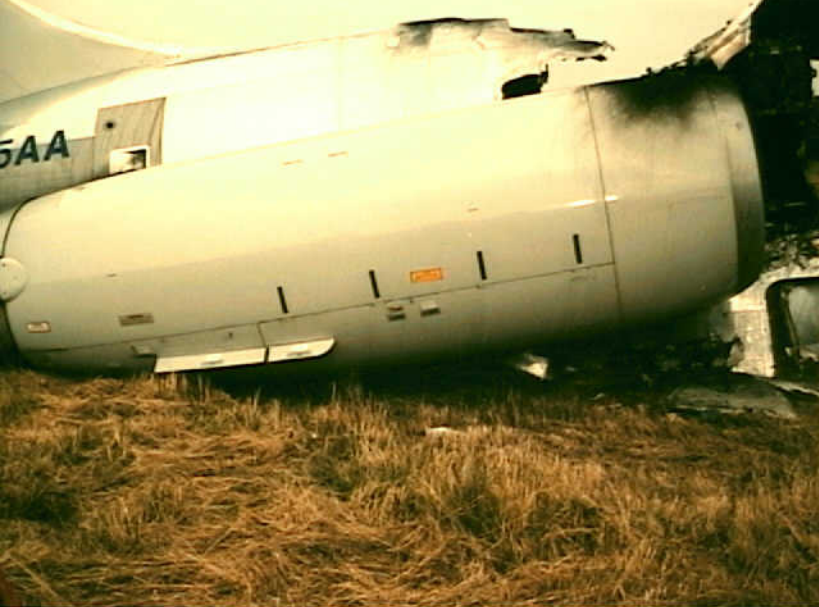
Powerplants 8 - Exhibit No. 8B - Photo 11. Left side of No. 1 engine thrust reverser in deployment position showing damage.
