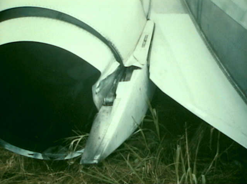
Powerplants 8 - Exhibit No. 8B - Photo 10. Close up of No. 2 engine fuel control in reverse thrust range.
