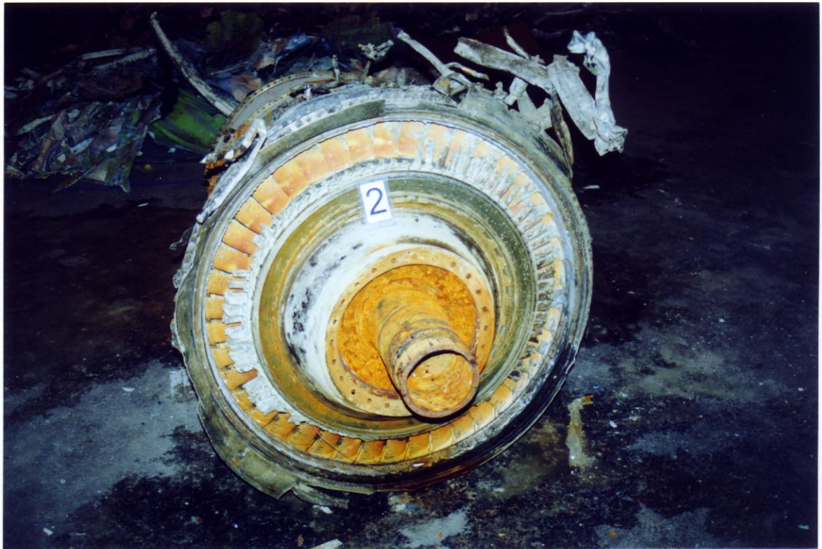
Photo 20. View of rear of No. 2 engine HPT.
