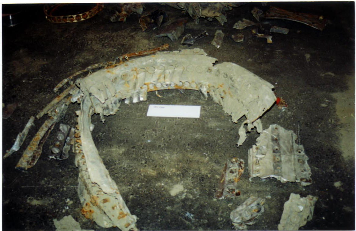
Photo 13. View of No. 2 engine HPC case showing variable stator vanes bent rearward.
