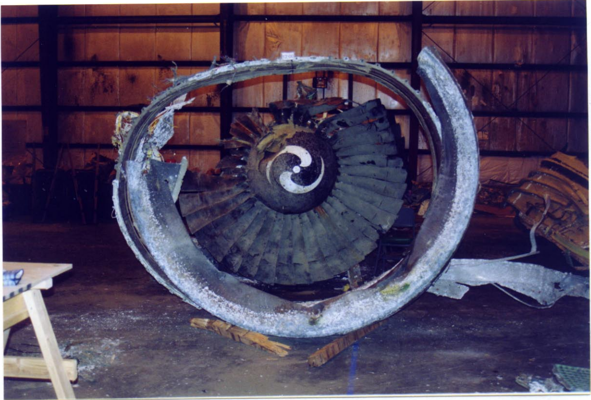
Photo 1. Front view of No. 1 engine inlet, fan containment case, and fan blades.
