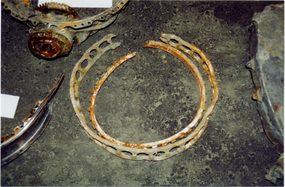
Photo 25. View of No. 2 engine No. 1 bearing cage.
