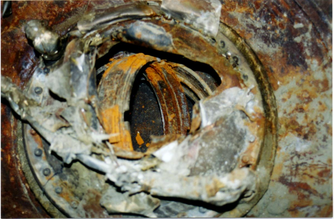
Photo 27. View of No. 2 engine No. 4 bearing outer race showing no rotational distress.
