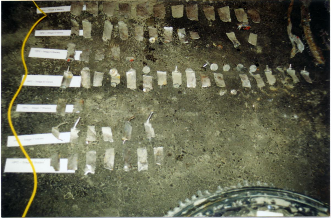
Photo 16. Pieces of No. 2 engine HPC blades and vanes.
