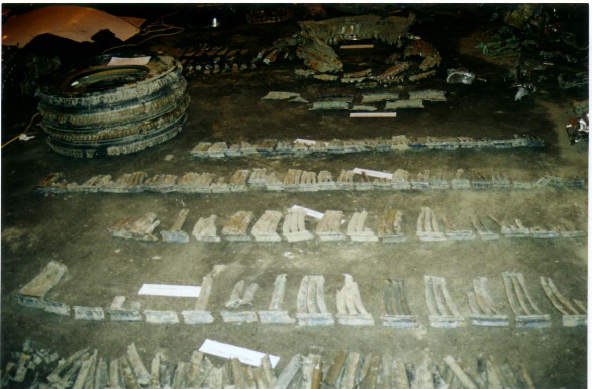
Photo 23. No. 2 engine LPT vanes showing straight airfoils and random lengths.
