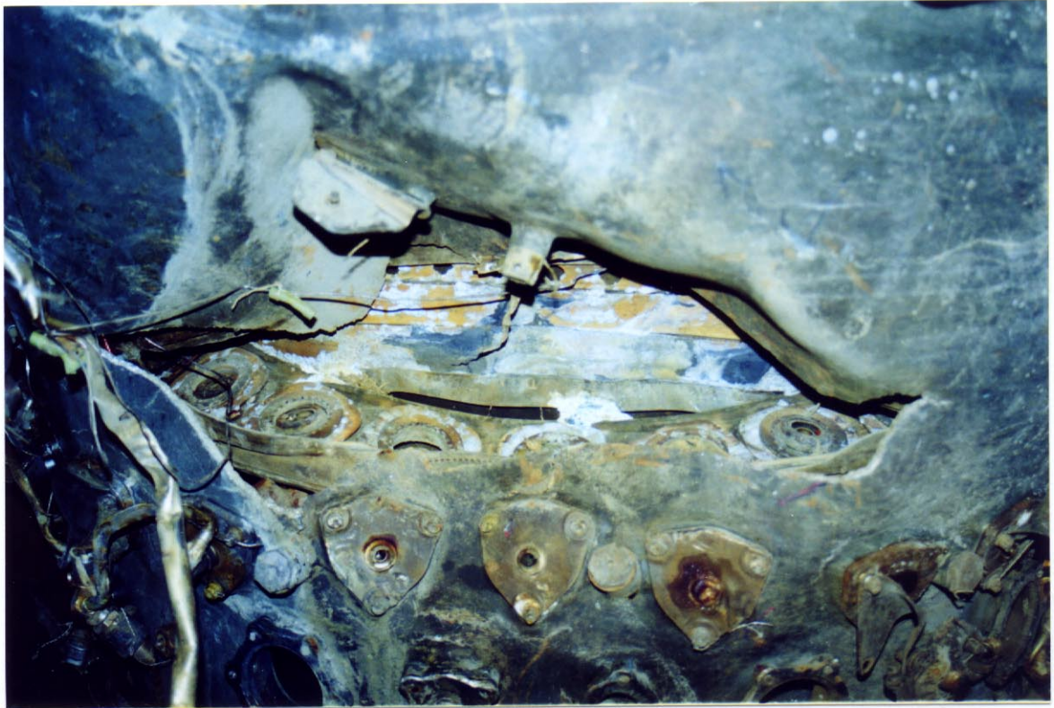
Photo 19. Closeup of hole in No. 2 engine combustor case showing no thermal distress to fuel nozzles and combustor liner.
