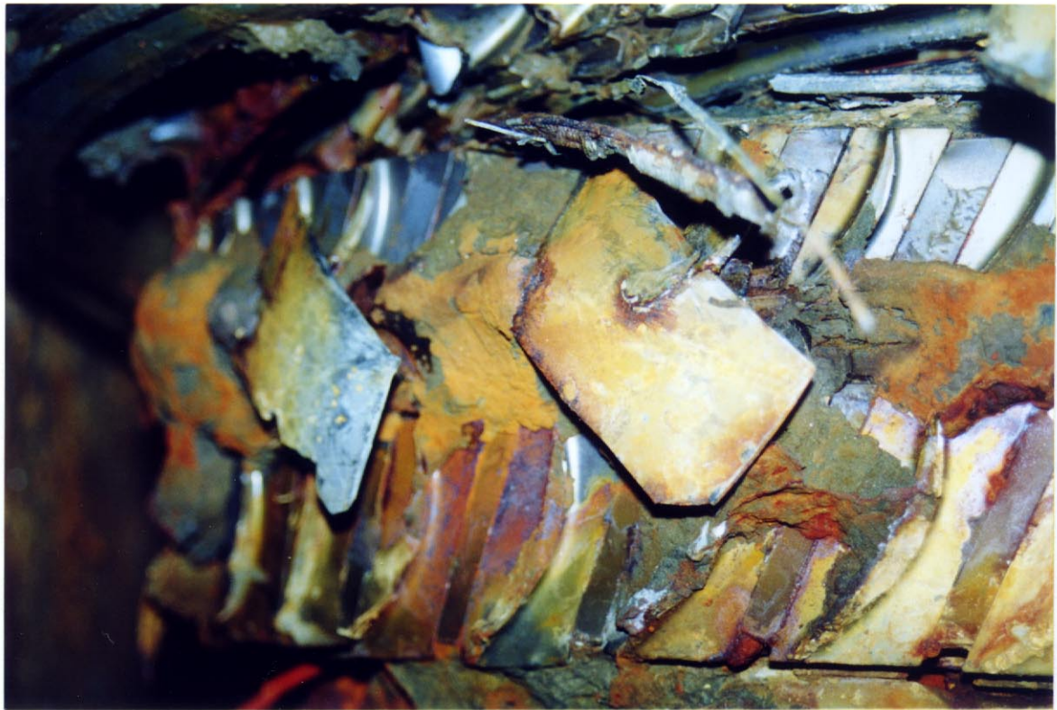
Photo 15. Closeup of No. 2 engine HPC blades showing no spanwise marks.
