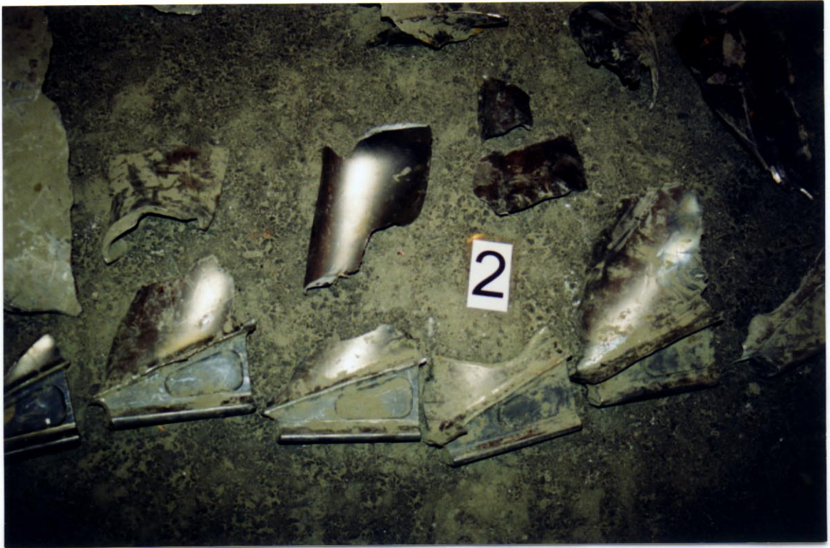
Photo 10. Pieces of No. 2 engine fan blades.
