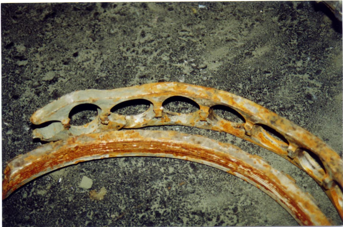
Photo 26. Closeup view of No. 2 engine No. 1 bearing cage pockets showing no rotational distress.
