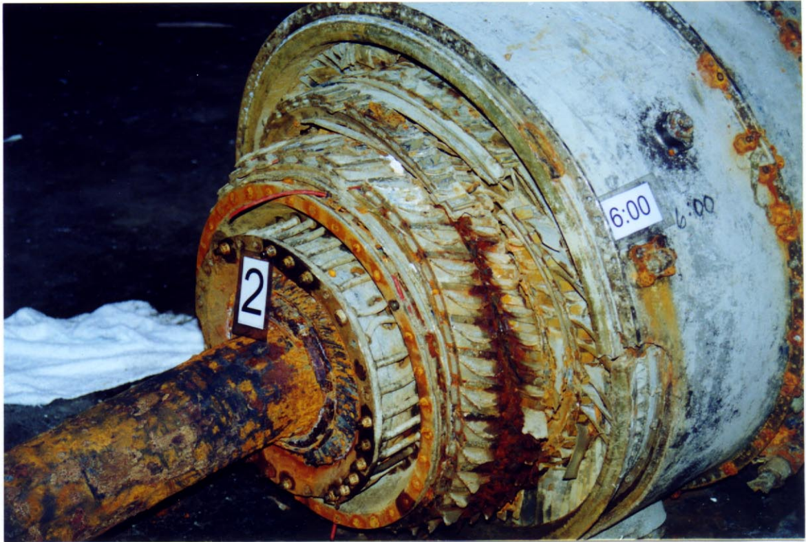
Photo 14. View of No. 2 engine HPC showing broken HPC disks and blades.
