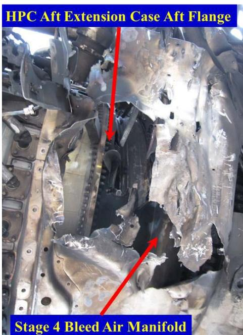
**PHOTO 39: HPC AFT EXTENSION CASE BREACH AT BOTTOM OF ENGINE**
