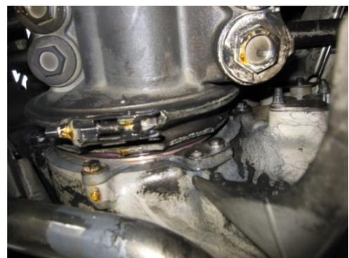
**PHOTO 31: FRACTURED LUBE AND SCAVENGE PUMP ATTACHMENT FLANGE**
