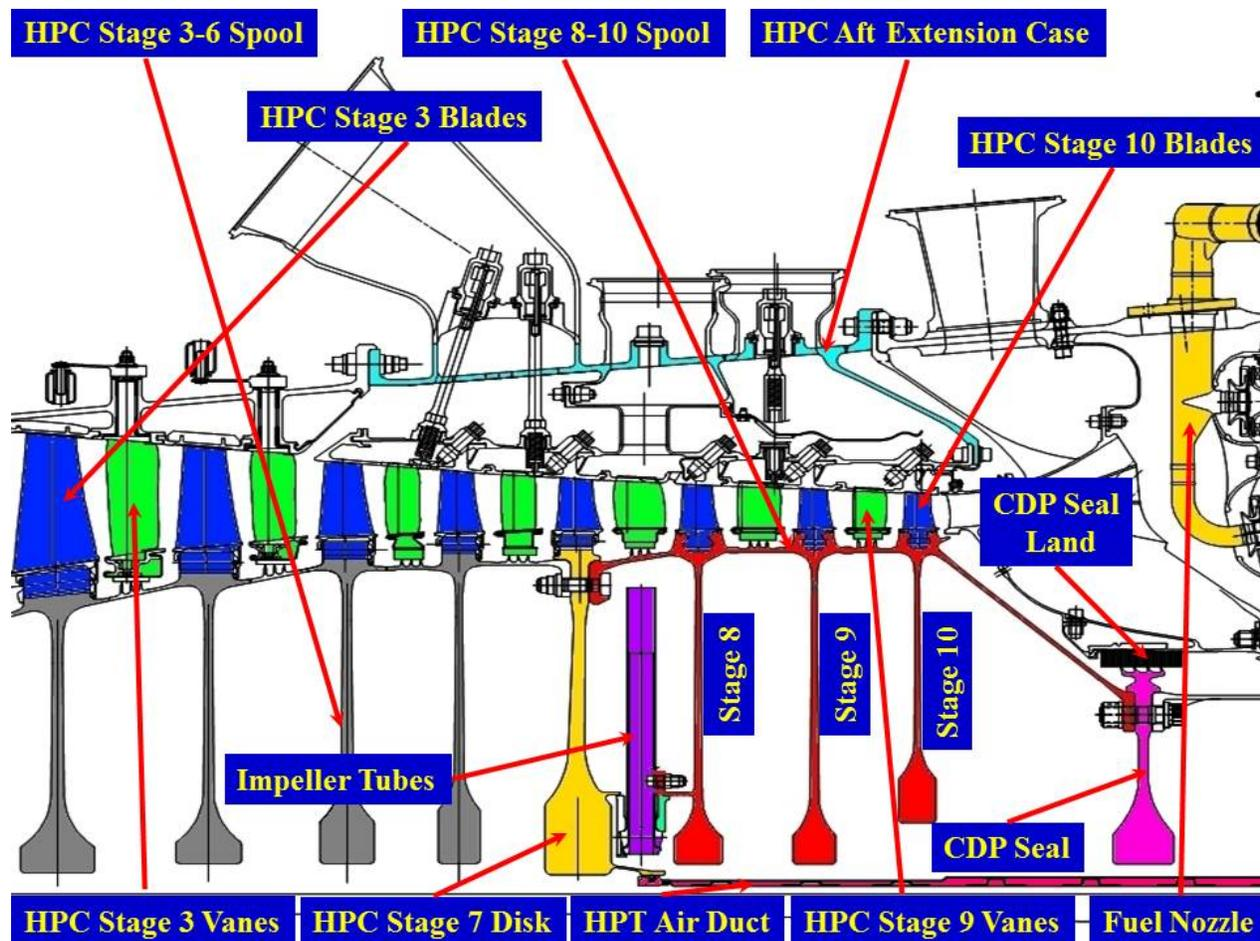
**FIGURE 5: CROSS-SECTION OF HIGH PRESSURE COMPRESSOR FOCUSED ON HPC STAGE 8-10 SPOOL<sup>8</sup>**
