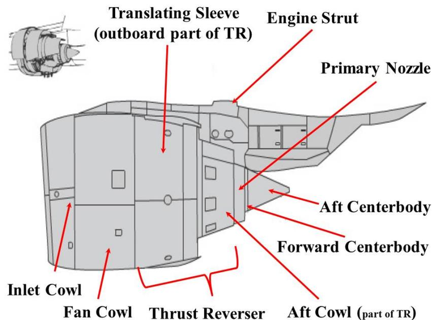
**FIGURE 3: BOEING 777 NACELLE NOMENCLATURE AND LOCATION**
