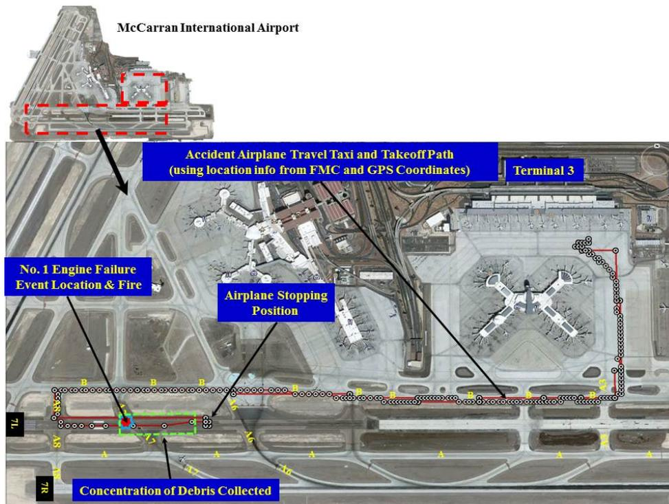
**FIGURE 4: AIRPORT DIAGRAM WITH AIRPLANE PATH AND DEBRIS LOCATIONS**
