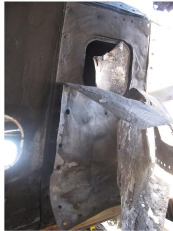
**PHOTO 24: MELTED & OPEN PRESSURE/RELIEF AND FIRE DETECTOR ACCESS PANEL**
