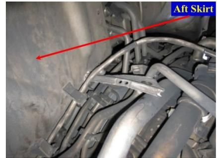
**PHOTO 34: ENGINE HEATSHIELD AFT SKIRT – AFT SIDE**
