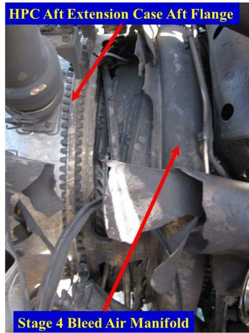
**PHOTO 38: HPC AFT EXTENSION CASE BREACH AT 3:00 O'CLOCK POSITION**
