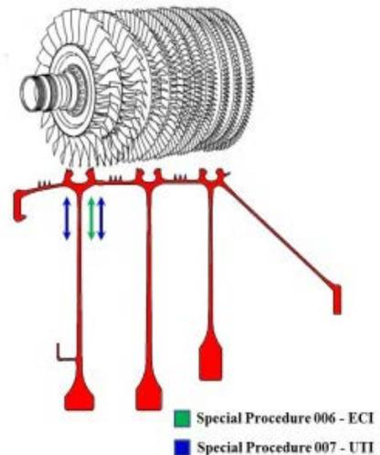
**FIGURE 14: ROTOR LEVEL SPECIAL PROCEDURE ECI AND UTI LOCATIONS**
