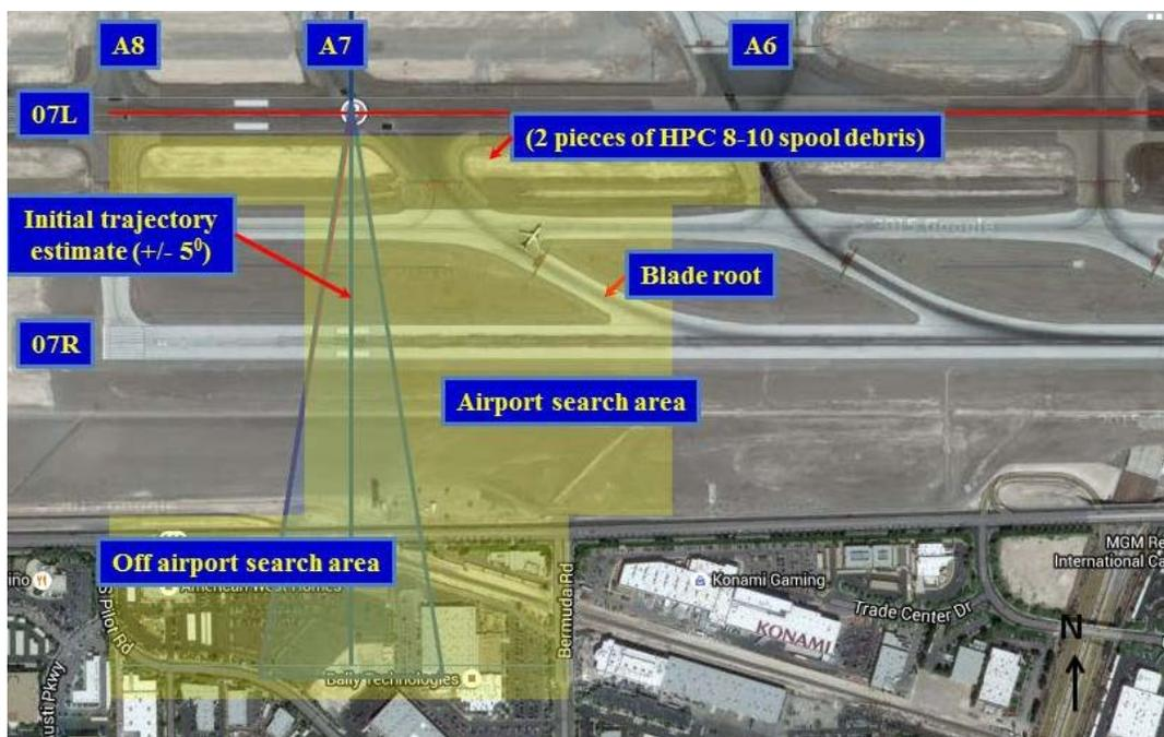
**FIGURE 7: PRELIMINARY TRAJECTORY PATH, SEARCH AREA, AND PARTS RECOVERED LOCATION**
