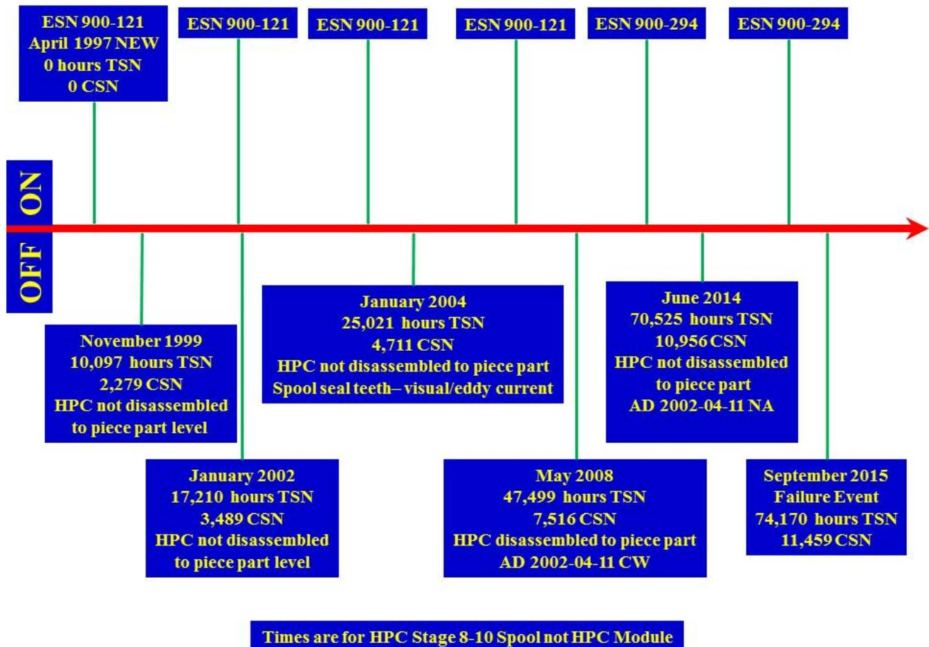
**FIGURE 2: TIMELINE OF HPC STAGE 8-10 SPOOL, PN 1694M80G04 AND SN GWNHA236**
