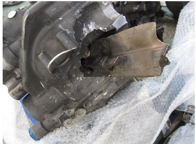
**PHOTO 36: HPC AFT EXTENSION CASE LODGED IN THE HMU**
