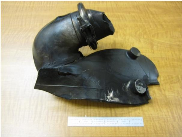
**PHOTO 13: HPC STAGE 7 BLEED AIR DUCT AND CASE PIECE FOUND WEDGED IN RIGHT TR TRANSLATING SLEEVE**
