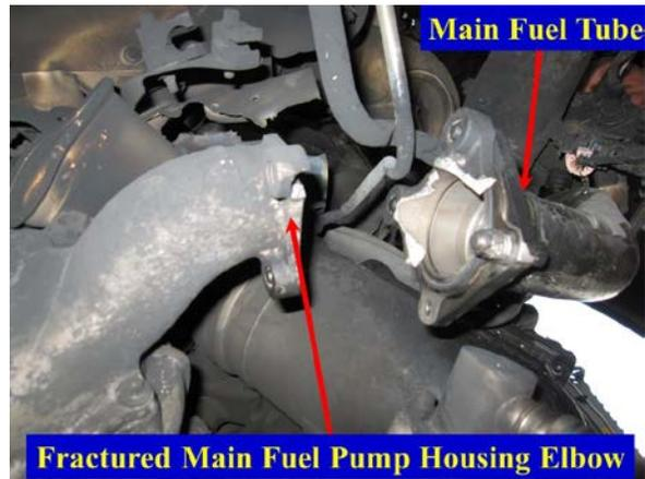
**PHOTO 29: MAIN FUEL SUPPLY LINE SEPARATED FROM THE MAIN FUEL PUMP**
