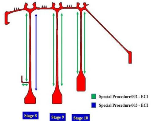
**FIGURE 13: PIECE PART SPECIAL PROCEDURE ECI LOCATIONS**
