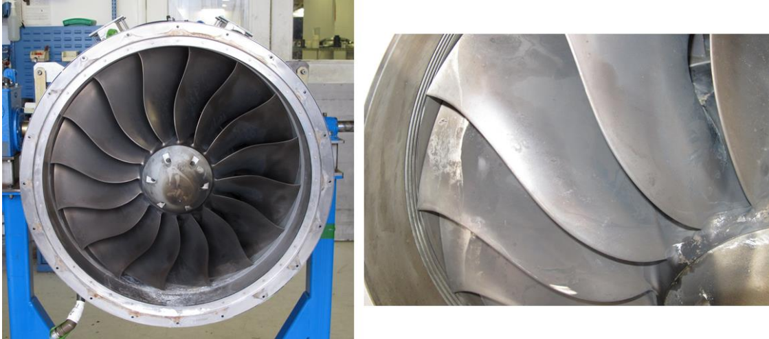
Photo 3- Fan Blade Sooting and Surface Deposits
