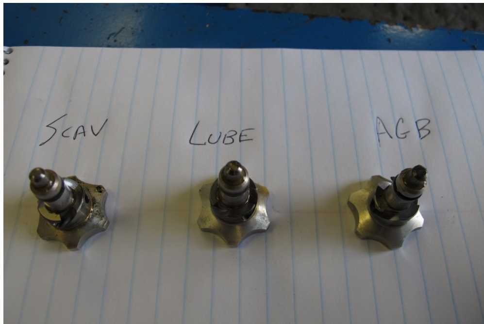
Photo 6- Chip Detectors, Free of Debris
