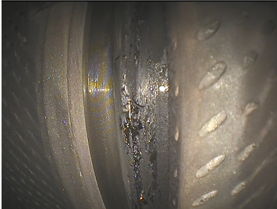
Photo 11- Borescope Photo of Fuel Slinger
