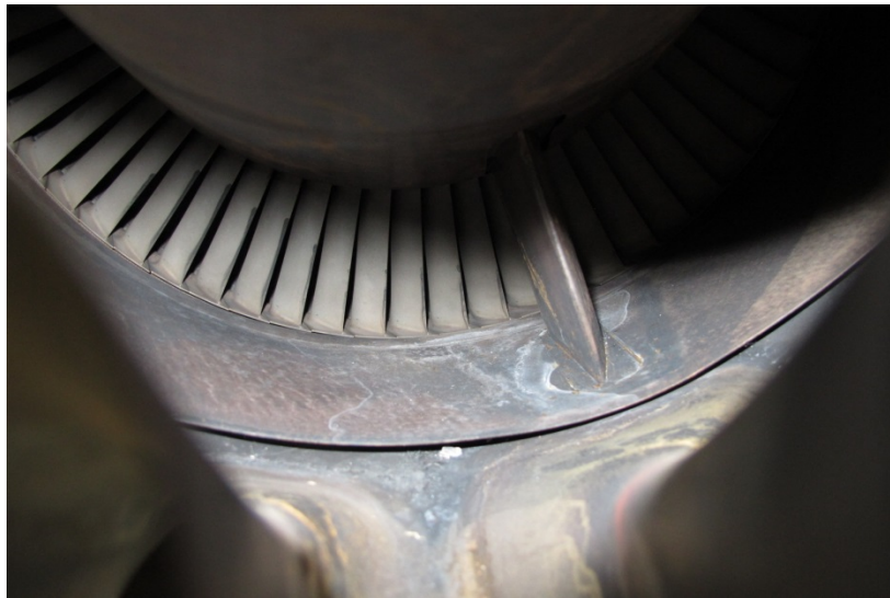
Photo 8- LPT 2 nd Stage Rotor Blades, Viewed Through the Exhaust
