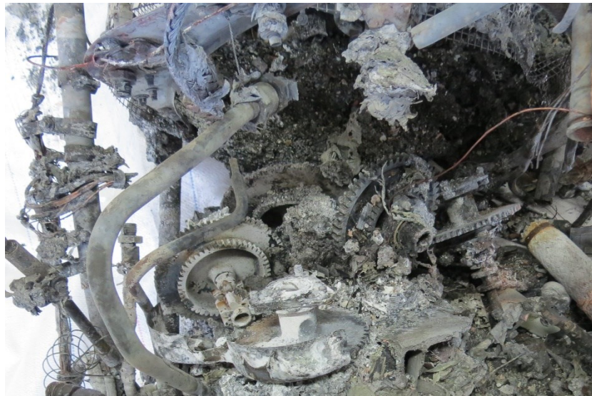
Figure 59. AGB components with thermally destroyed diaphragm and housing
