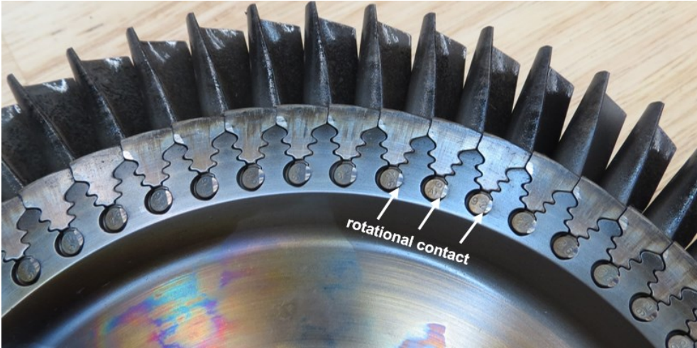
Figure 26. CT disk assembly upstream side showing rotational scoring along blade retention rivets and platforms
