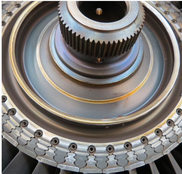
Figure 32. PT S2 disk assembly, downstream face
