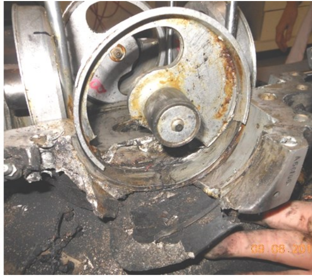
Figure 10. Fractured aft hub with D blade preload plate
