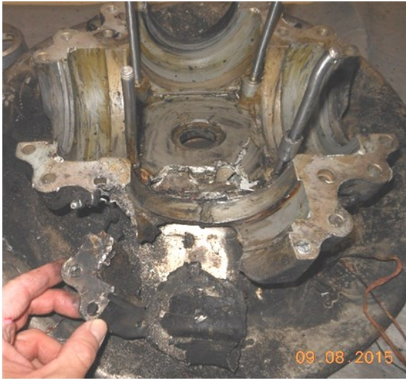
Figure 9. Aft hub fractured at D blade socket
