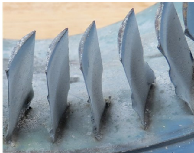
Figure 23. S1 compressor stator vanes
