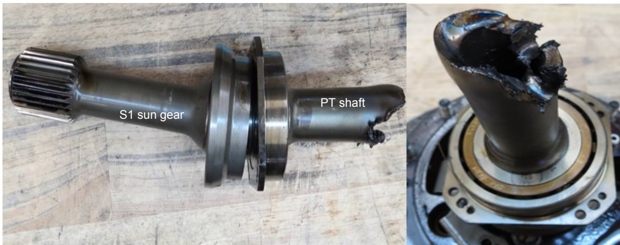
Figure 33. S1 sun gear and forward section of fractured PT shaft; detail of fracture surface
