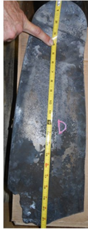
Figure 6. Blade section recovered from roof
