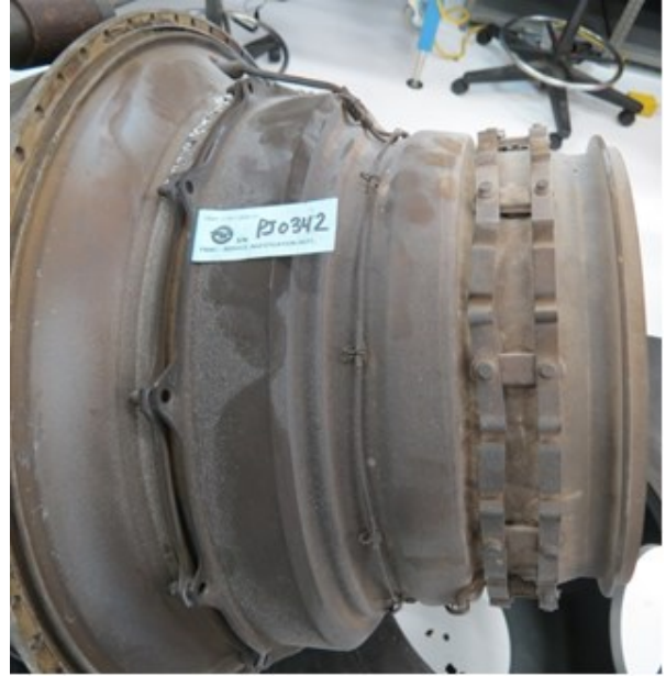
Figure 28. Failed PT housing flange attachment
