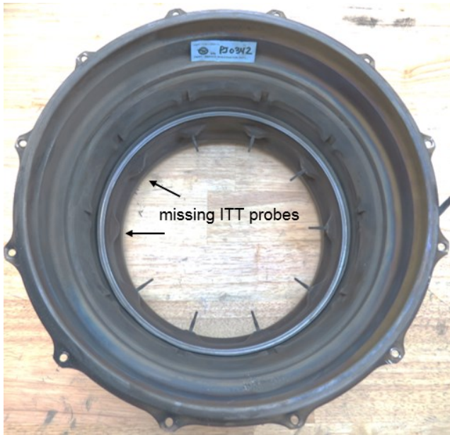
Figure 27. PT housing showing missing ITT probes
