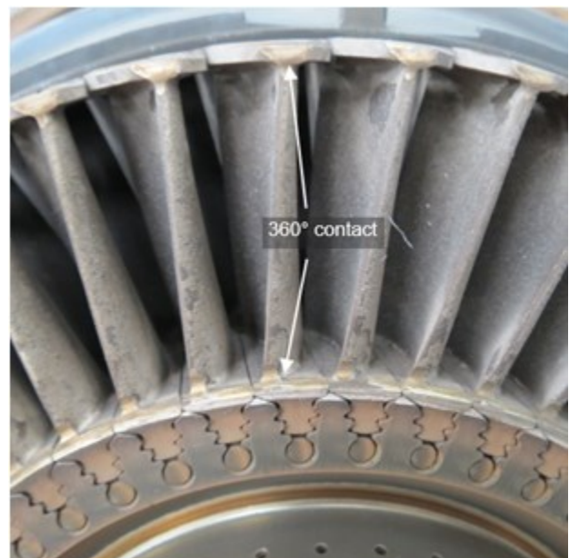
Figure 31. Upstream face of PT S1 disk assembly
