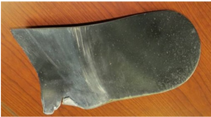
Figure 5. Views of blade tip section recovered from parking lot
