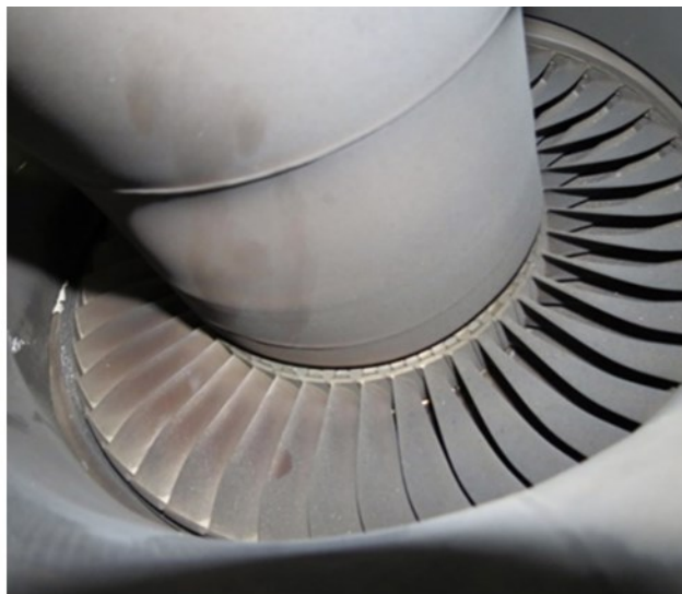
Figure 19. PT rotor viewed through the exhaust
