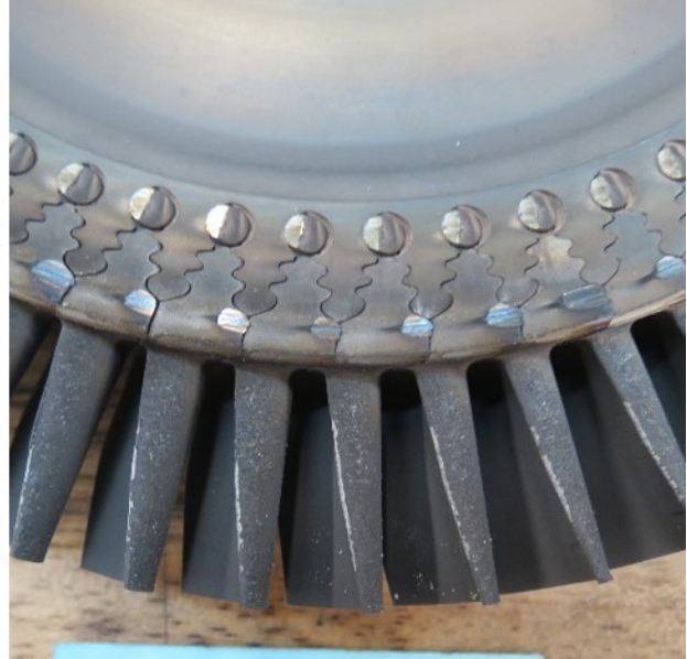
Figure 55. CT disk assembly upstream side
