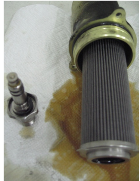
PHOTO 28: CLEAN OIL MAGNETIC CHIP DETECTOR AND OIL FILTER
