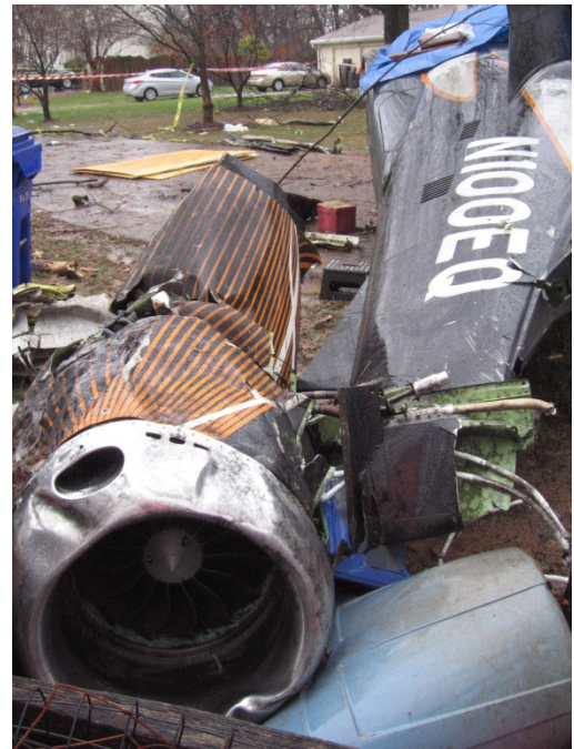
PHOTO 3: NO. 1 ENGINE IN-SITU (RESTING NEAR THE EMPENNAGE)
