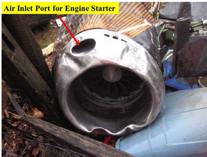
PHOTO 4: INLET NOSE COWL WITH ROUND- BOTTOM IMPACT DAMAGE
