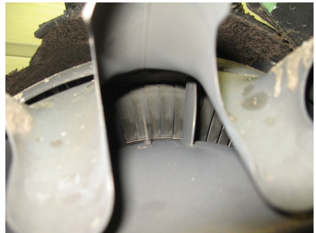
PHOTO 20: LPT BLADES INTACT AND GOOD CONDITION
