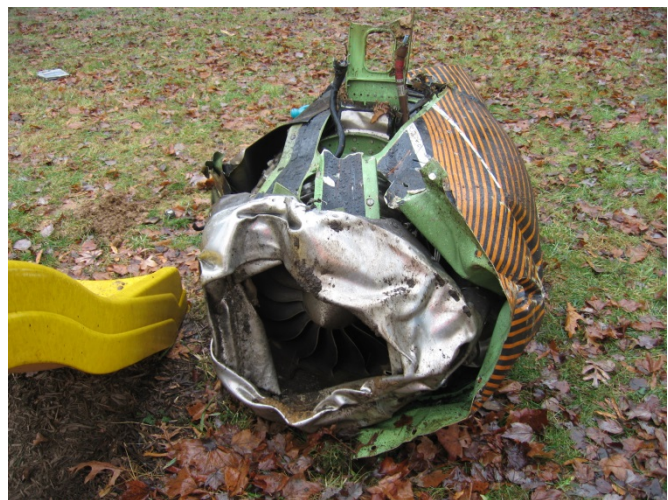
PHOTO 8: INLET COWL WITH SEVERAL ROUND-BOTTOM IMPACTS
