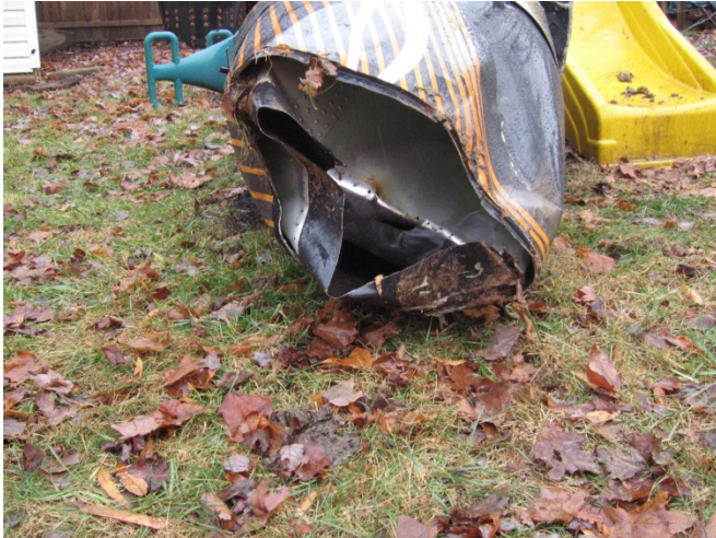
PHOTO 9: DISTORTED EXHAUST PIPE
