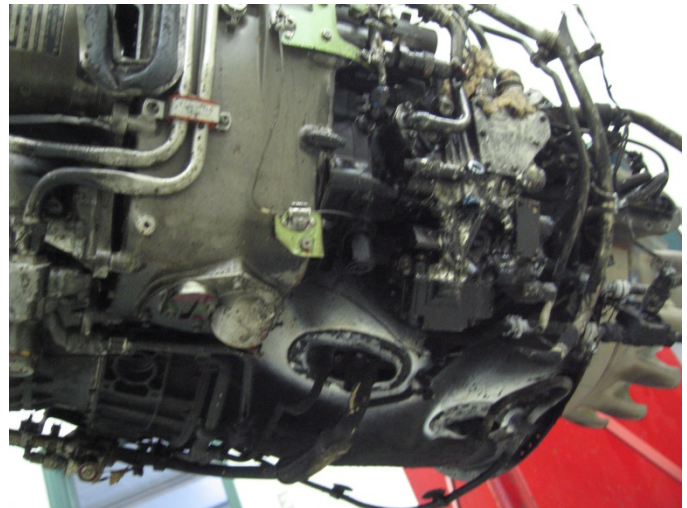
PHOTO 26: THERMAL DISTRESS AND IMPACT DAMAGE
