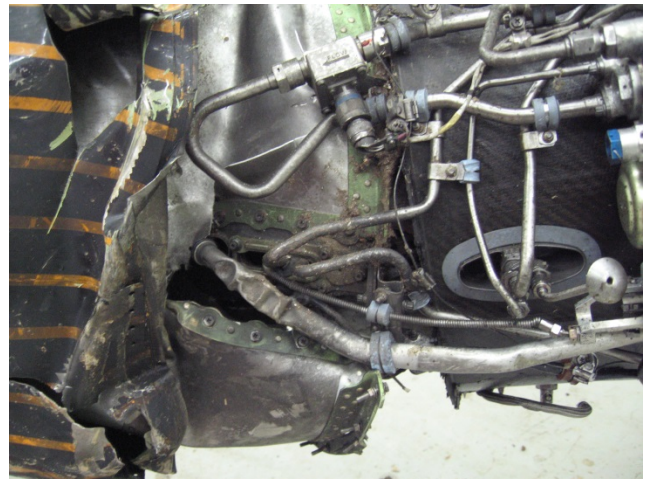
PHOTO 18: SEPARATED BYPASS DUCT (BOTTOM VIEW WITH PIPING STILL ATTACHED)
