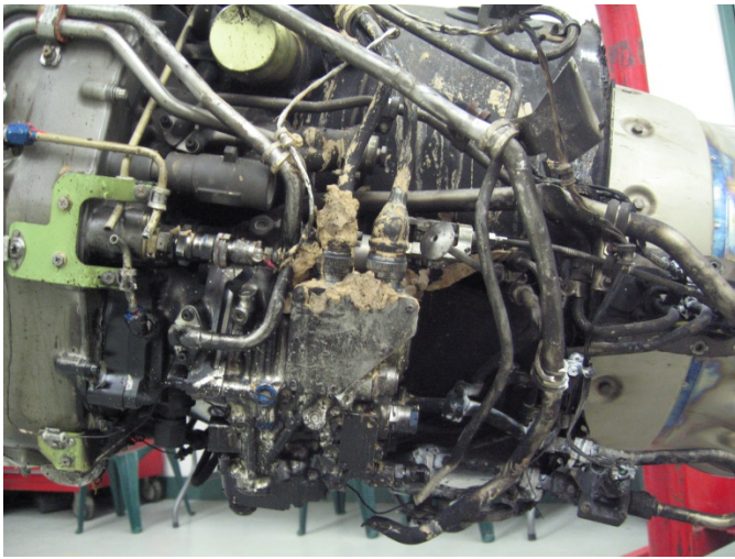
PHOTO 25: THERMAL DISTRESS AND IMPACT DAMAGE
