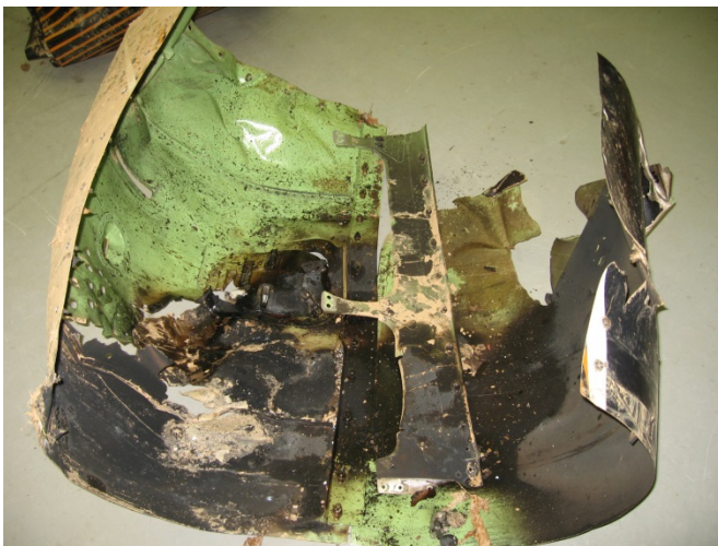
PHOTO 23: COWLING THERMAL DAMAGE
