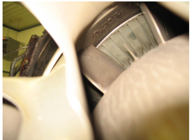
PHOTO 30: LPT BLADES INTACT AND GOOD CONDITION
