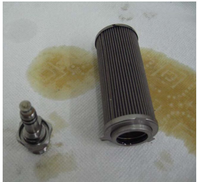
PHOTO 16: CLEAN OIL MAGNETIC CHIP DETECTOR (LEFT) AND OIL FILTER (RIGHT)
