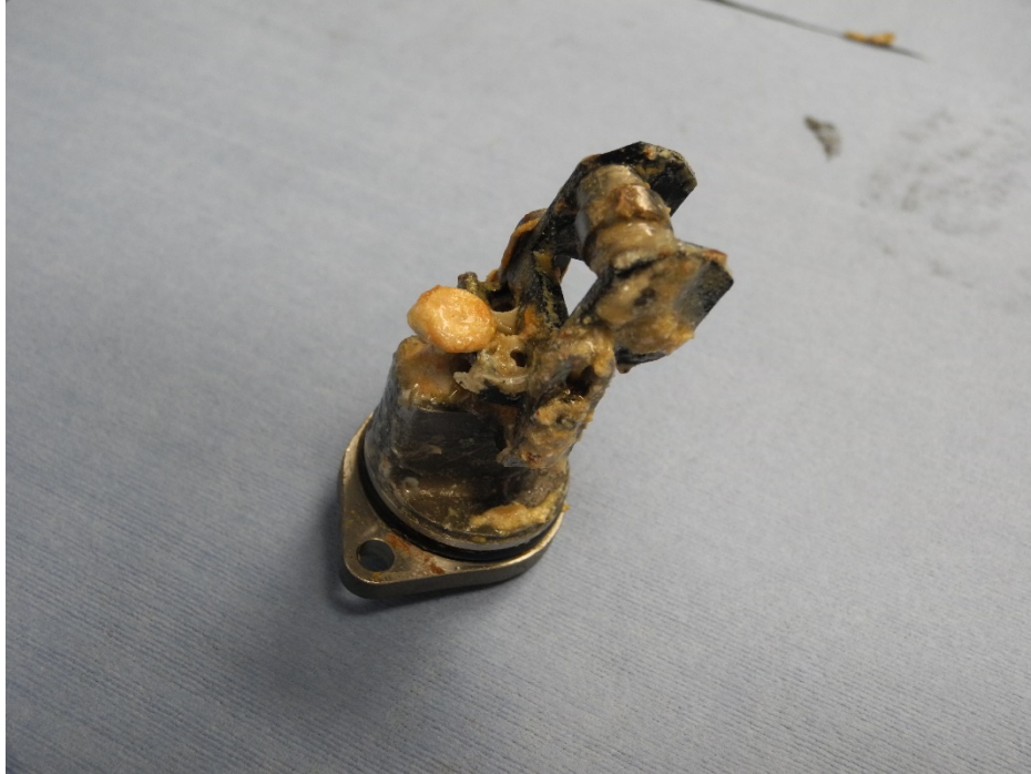
Photo 33 – Slope Stop Assembly - Undamaged
