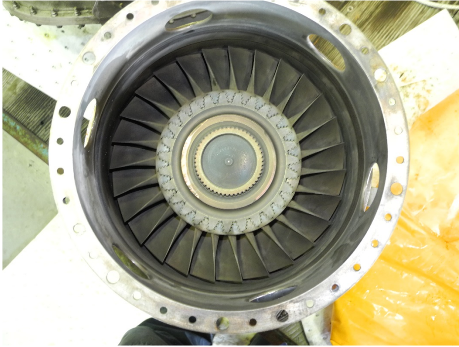
Photo 15 – Power Turbine Blades – Leading Edges and Pressure Side Chords - Undamaged
