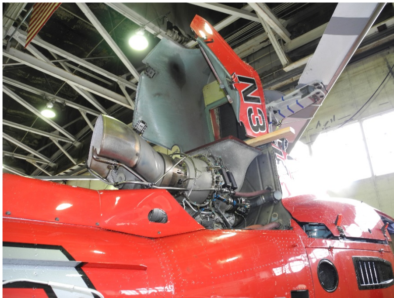
Photo 2 - N350LH Engine Cowling Raised
