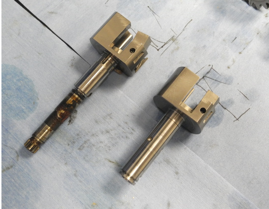
Photo 37 – Nf & Ng Flyweight Assemblies - Undamaged
