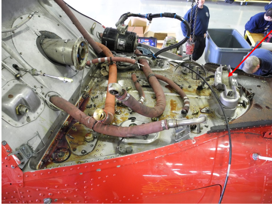
Photo 11 – Engine Bay After Removal of Engine – Undamaged
