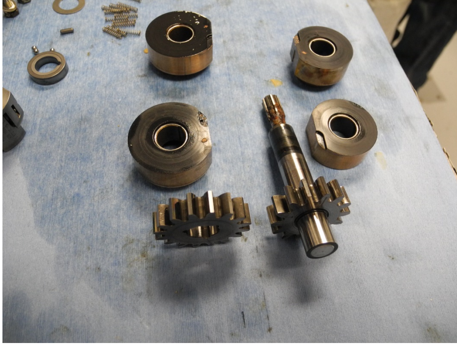
Photo 41 – Fuel Pump Gears & Side Seals - Undamaged
