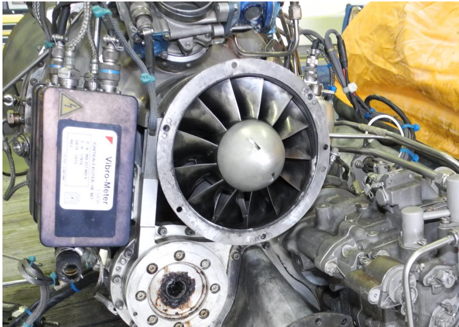
Photo 20 – 1 st Stage Compressor Wheel - Undamaged
