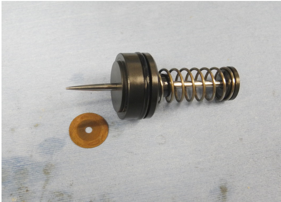
Photo 36 – Main Metering Valve – Clean and Undamaged
