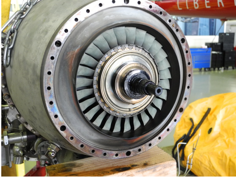
Photo 19 - 2 nd Stage GG Turbine - Undamaged
