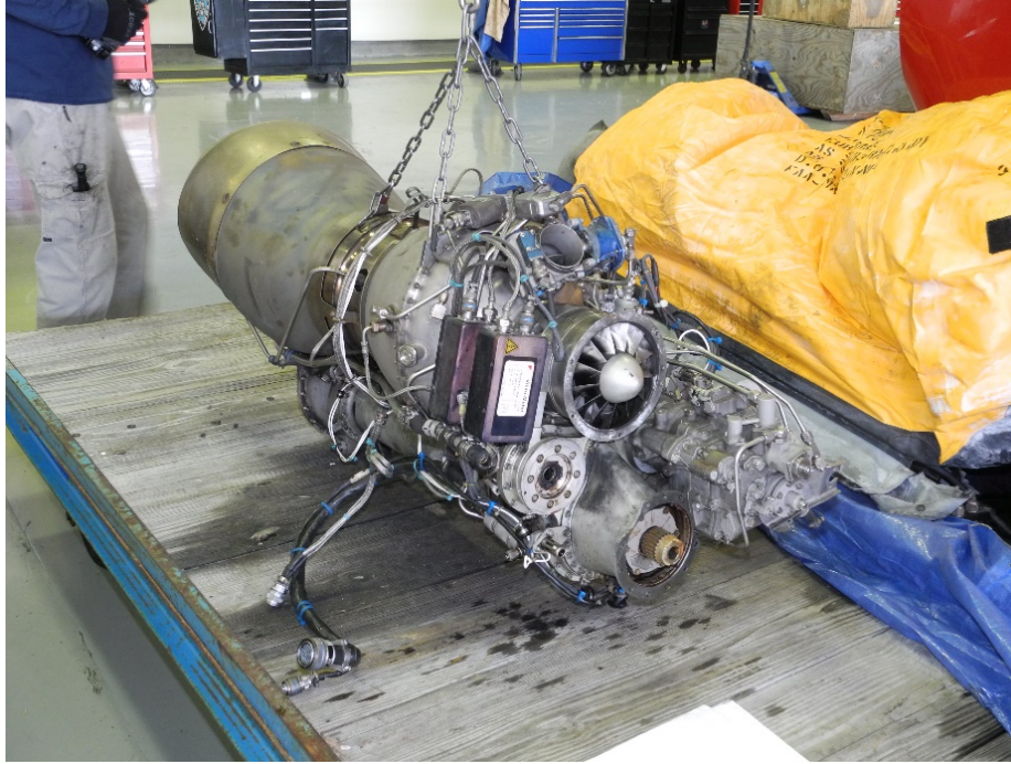
Photo 9 – Engine Removed from the Helicopter
