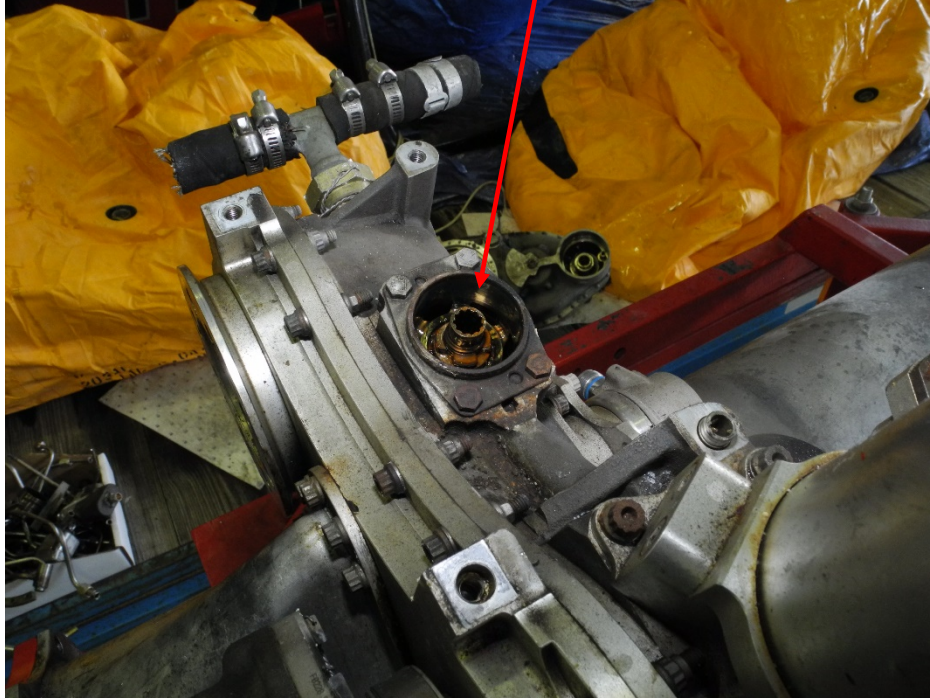
Photo 21 - Bevel Gear Input Spline - Undamaged
