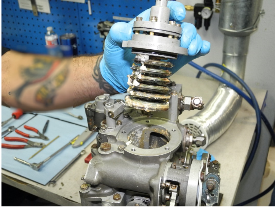
Photo 27 – Acceleration Controller Cavity – Water/Grease Mixture
