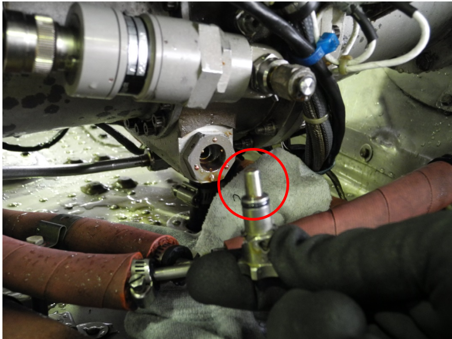
Photo 4 – Manual Magnetic Chip Plug from Module 01 (AGB) - Clean
