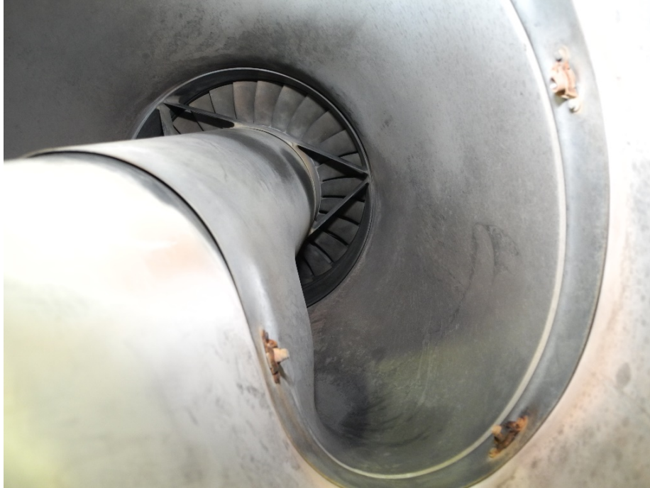
Photo 3 – Power Turbine Blades – Undamaged
