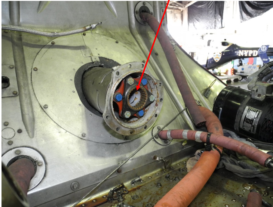
Photo 10 – Transmission Input Shaft Spline - Undamaged
