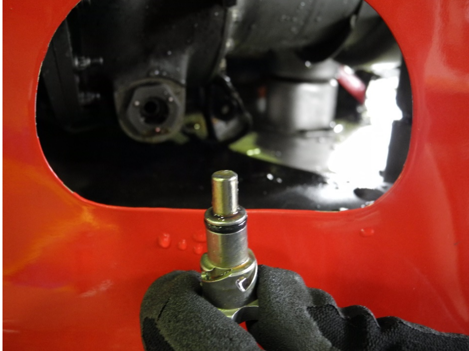
Photo 5 – Manual Magnetic Chip Plug from Module 05 (RGB) - Clean
