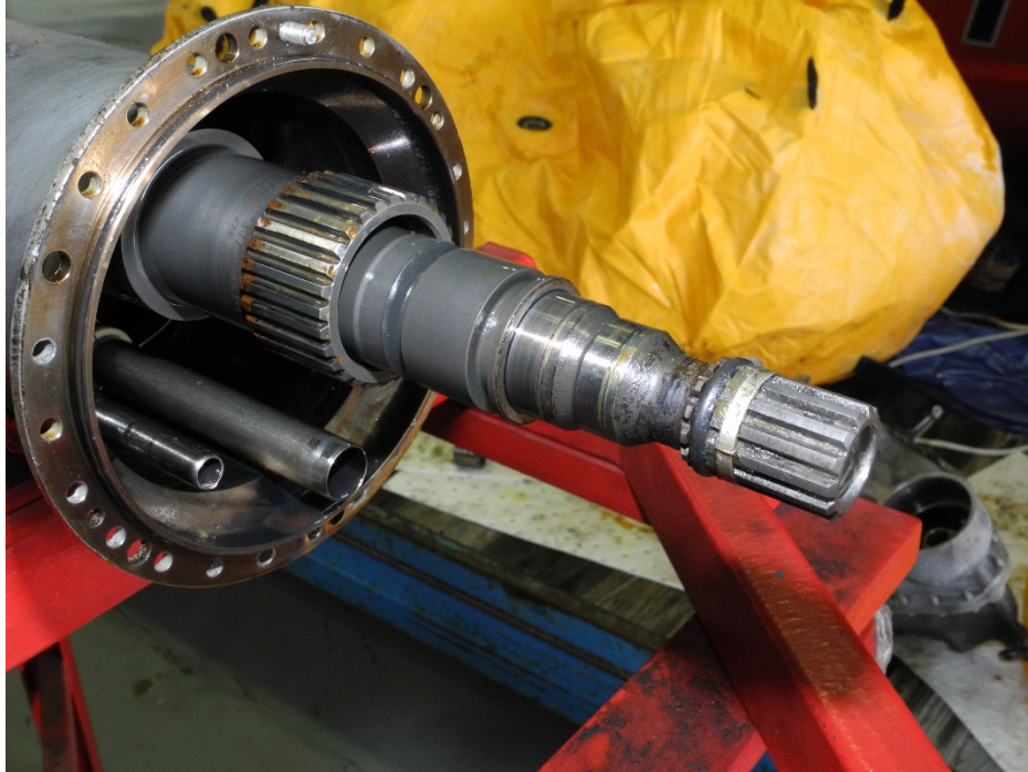
Photo 23 - Freewheel Shaft Spline - Undamaged
