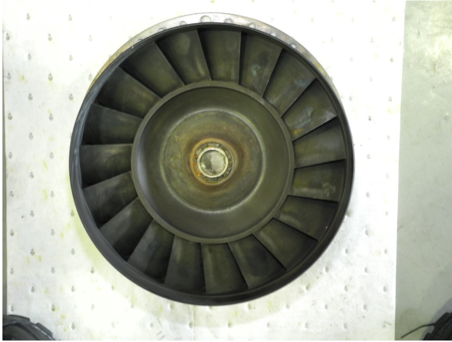
Photo 17 - Power Turbine Nozzle Guide Vane – Trailing Edges - Undamaged
