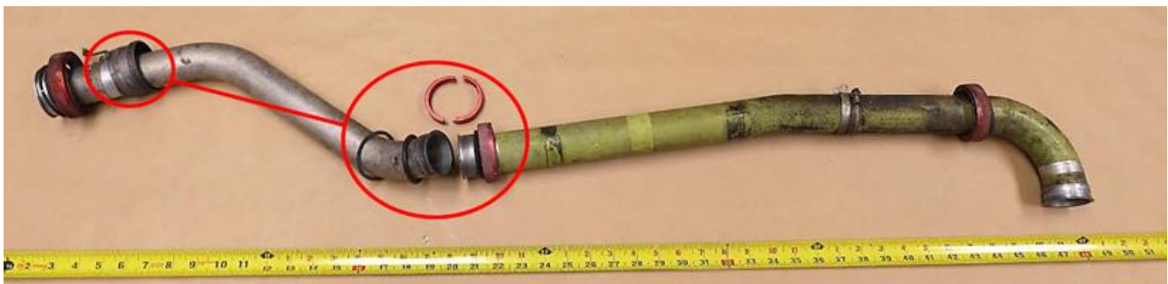
Photo 167- Left Engine Main Fuel Supply Lines and Fuel Coupling Assembly, as received at Boeing
