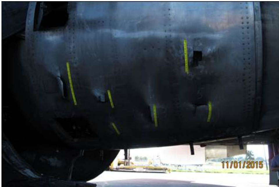
Photo 5- Core Cowl Thermal Damage, Outboard Side
