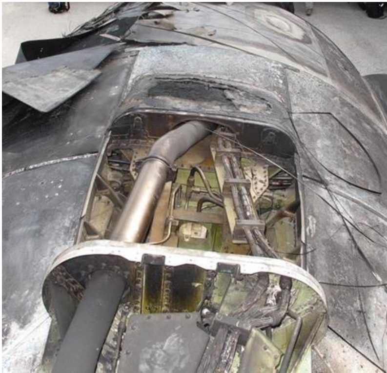
Photo 15- Upper Forward Strut Compartment
