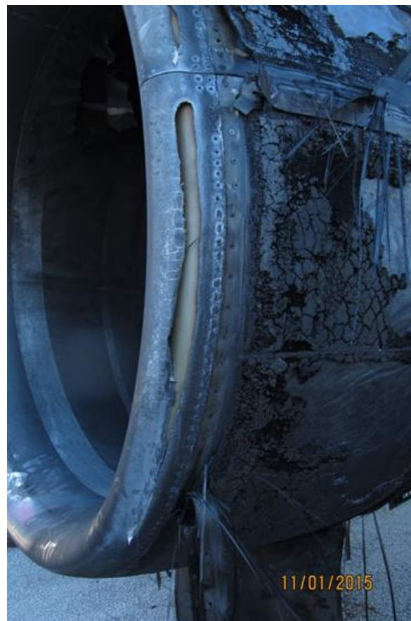
Photo 3- Inlet Cowl Forward Lip Thermal Damage
