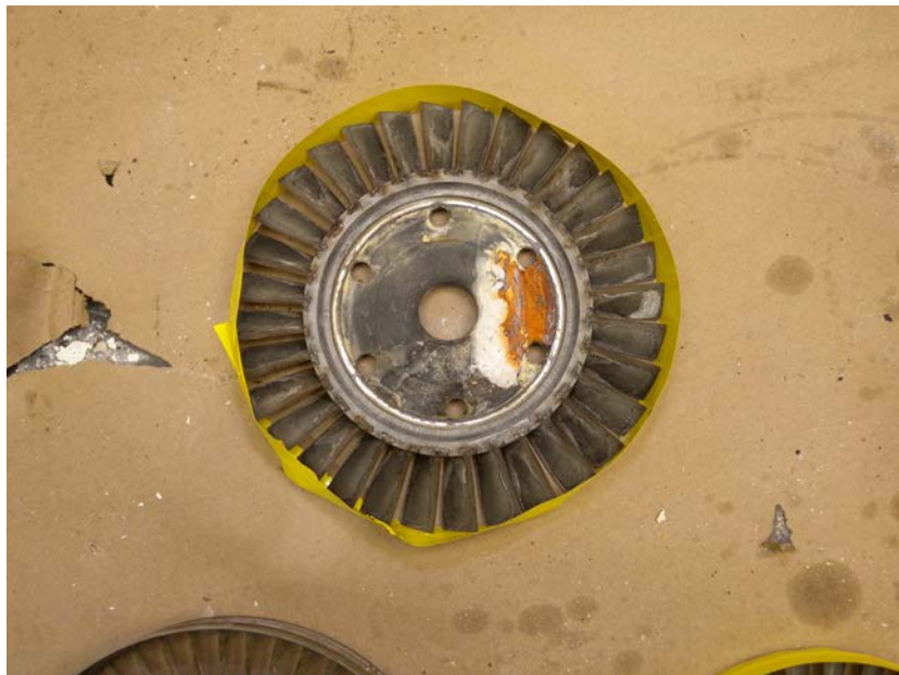
Figure 27 – 2 nd Stage Compressor Wheel
