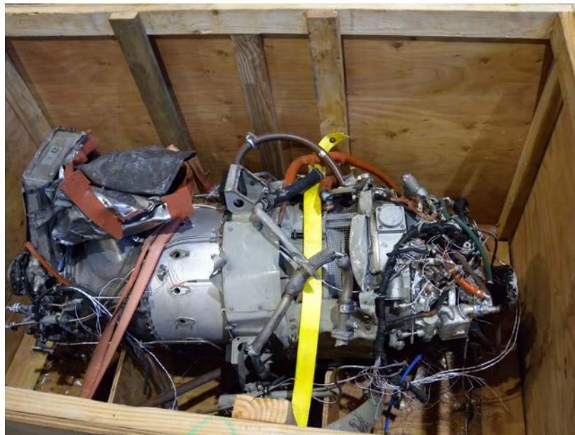
Figure 3 – PT6A-114A Engine S/N PCE-PC1021 – As Received
