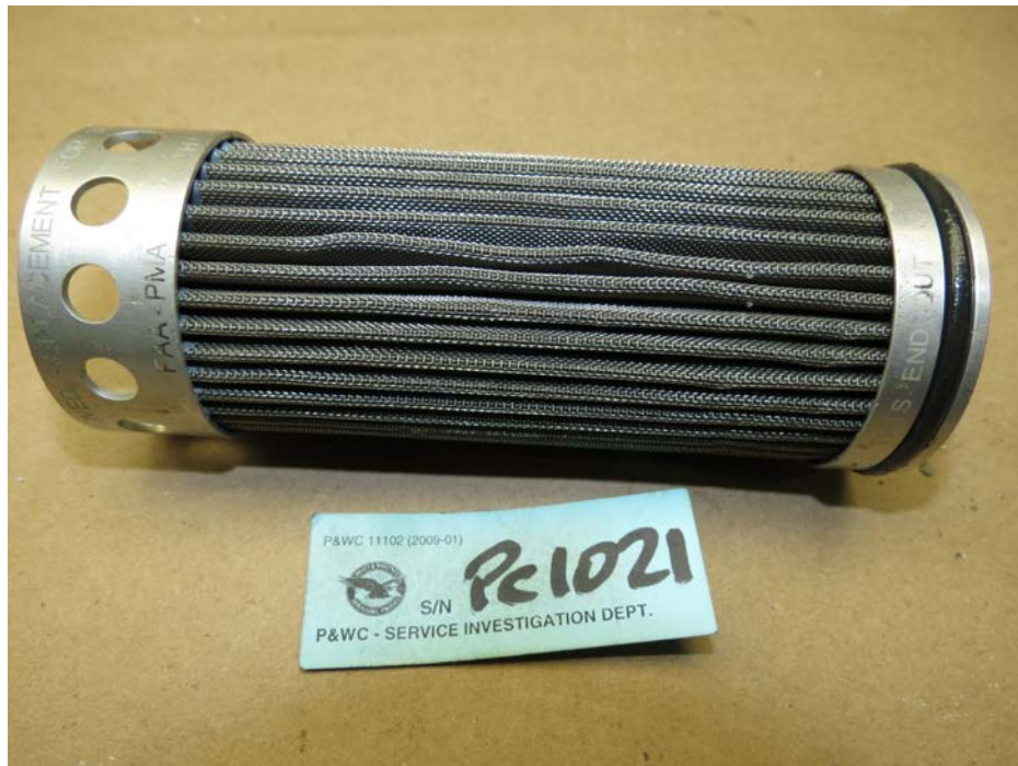
Figure 43 – Main Oil Filter – Clean, but Contained Water
