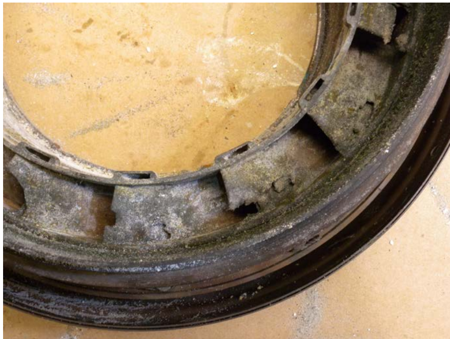
Figure 17 – Compressor Turbine Vane Ring – Trailing Edges - Detail
