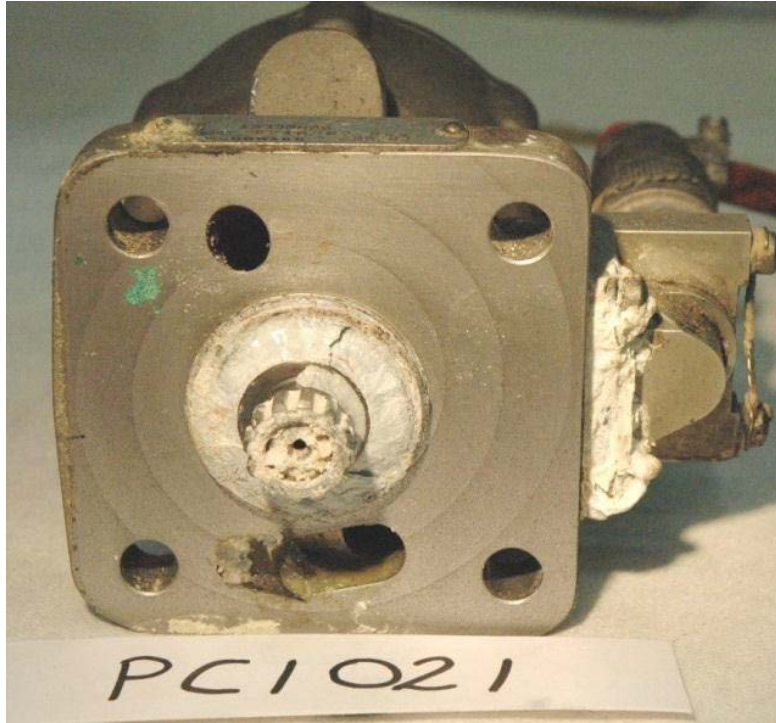
Figure 40 - Overspeed Governor - Driveshaft Cavity
