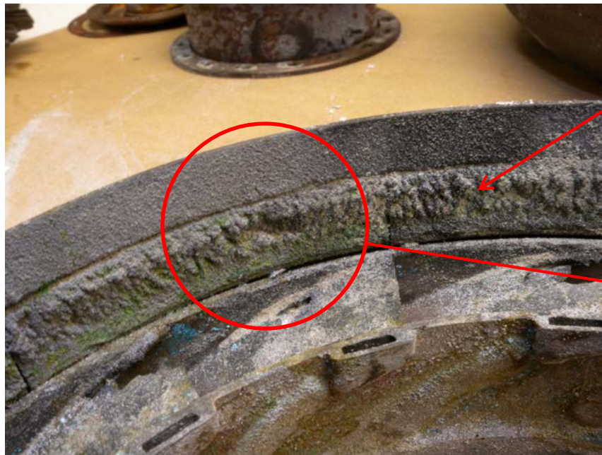
Figure 18 – Compressor Turbine Shroud – Detail at 4:00 O'clock
