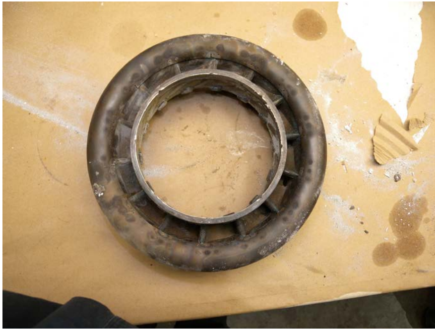
Figure 16 – Compressor Turbine Vane Ring – Front View
