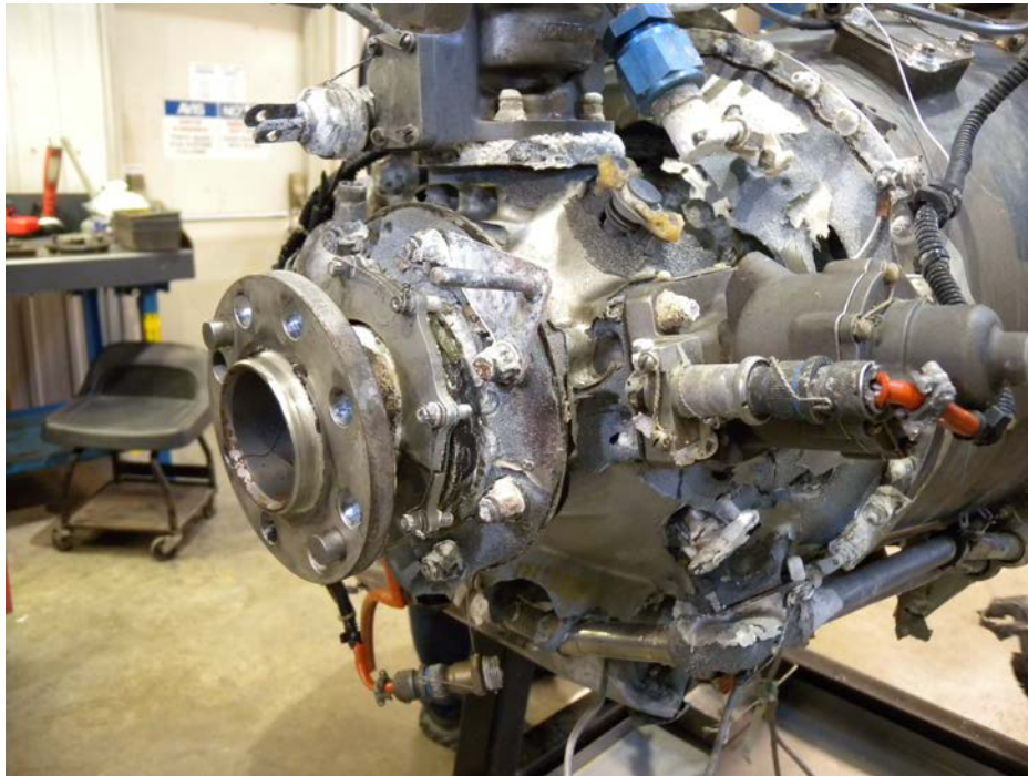
Figure 39 – Overspeed Governor – In Situ
