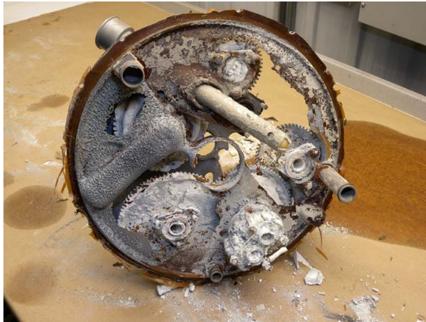
Figure 30 – Accessory Gearbox (AGB) – Dissolved, Exposing Internal Components
