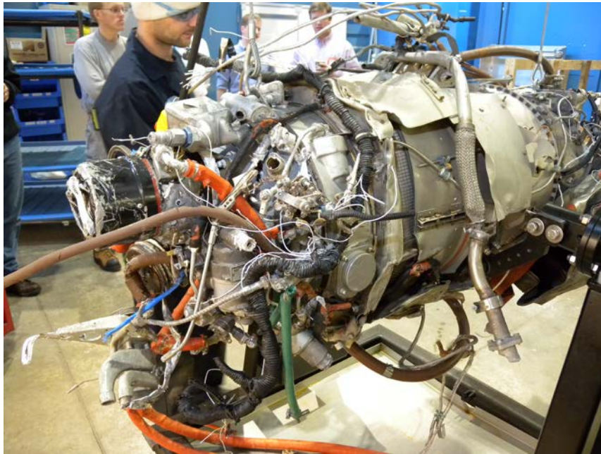
Figure 4 - PT6A-114A Engine S/N PCE-PC1021 - As Received
