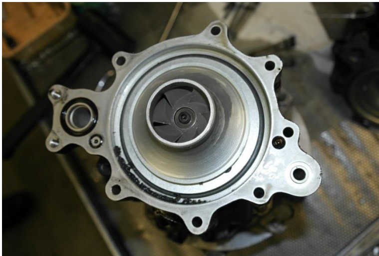
PHOTO 15: BLACK DEBRIS IN HYDRAULIC PUMP
