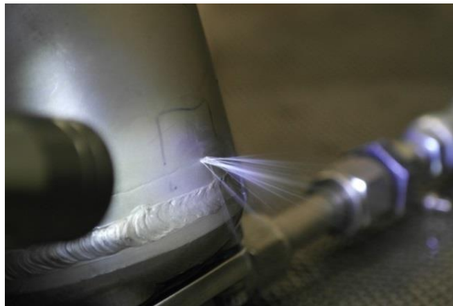
PHOTO 20: LEAK AT 250 PSI FLUID PRESSURE
