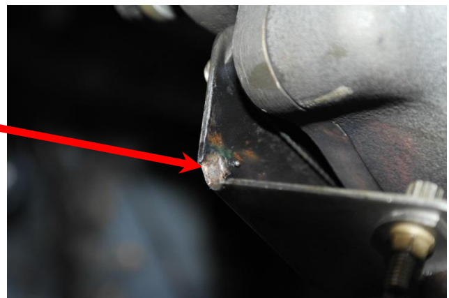
PHOTO 27: MOLTEN METAL ON AFT SIDE OF OIL LINE BRACKET
