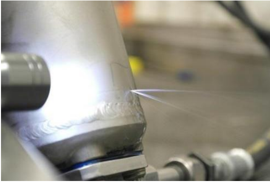
PHOTO 18: LEAK AT 10 PSI FLUID PRESSURE
