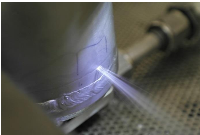
PHOTO 21: LEAK AT 400 PSI FLUID PRESSURE
