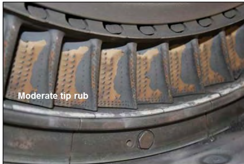
Figure 7: Images of the forward side (upper) and outboard side (lower) of the 1 st stage HPT blades
