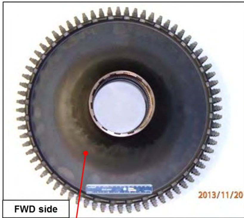
Oil wetting evident on FWD side of hub
