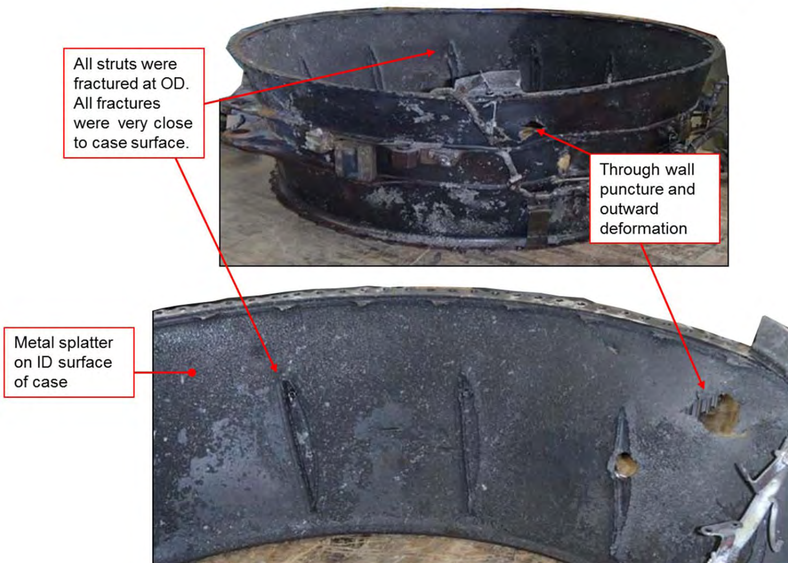
Figure 20: Images of the turbine exhaust case (TEC)
