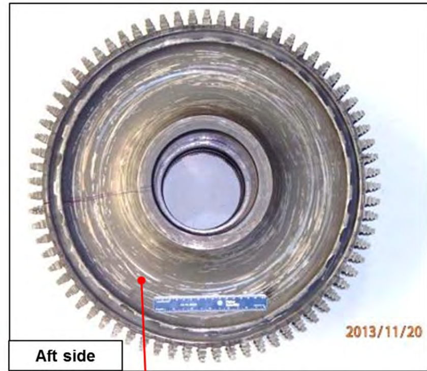
Mechanical damage evident on AFT side of hub
