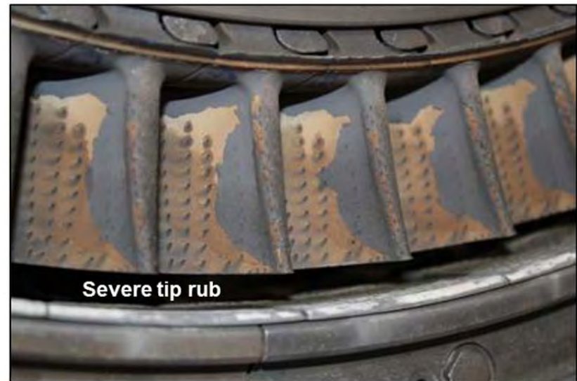
Figure 7: Images of the forward side (upper) and outboard side (lower) of the 1 st stage HPT blades
