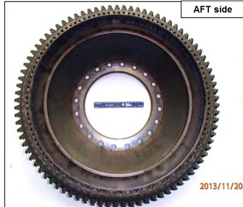
Figure 15: Overall images of the 6 th stage LPT disk
